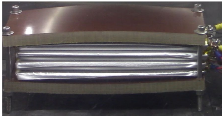
Figure 20. Still frame captured from the video of the 1s4p OC test
