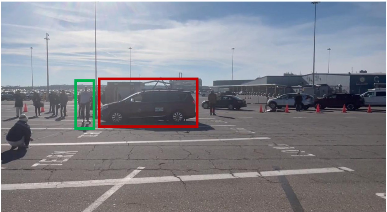
(b) Dummy pedestrian emerges; CP-enabled safe stop
