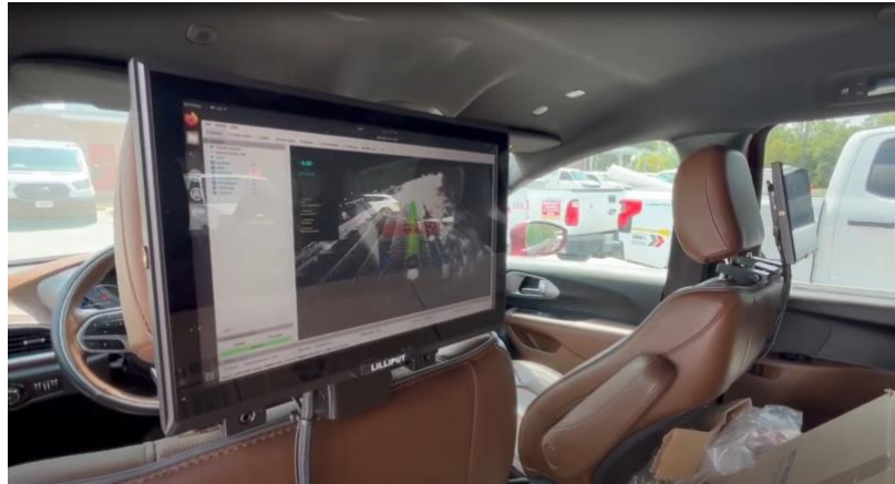
(b) Real-time Process of 3D point cloud from Lidar
