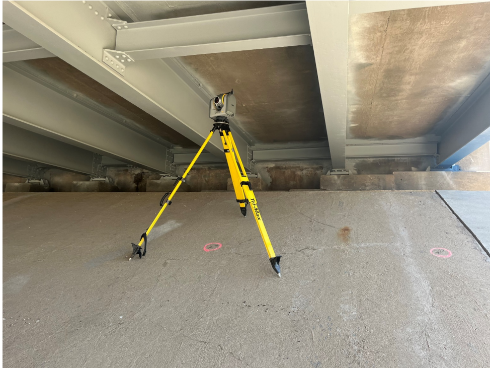
A. Scanner positioned on the slope wall. Control points are marked with pink paint.
