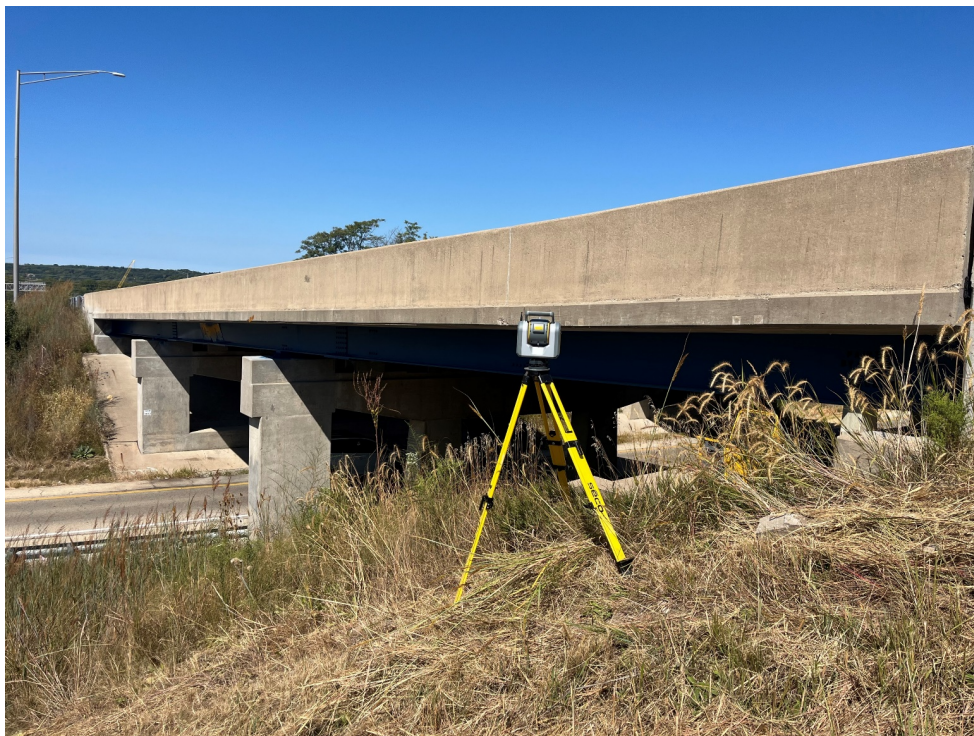
B. Scanner positioned on the approach embankment next to a bridge.
