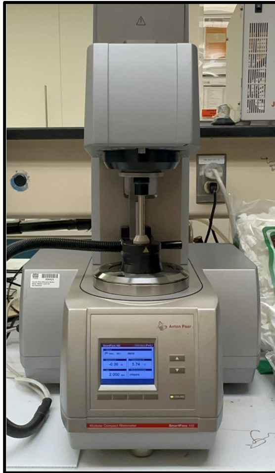
Figure 3.10. Dynamic Shear Rheometer used in this study
