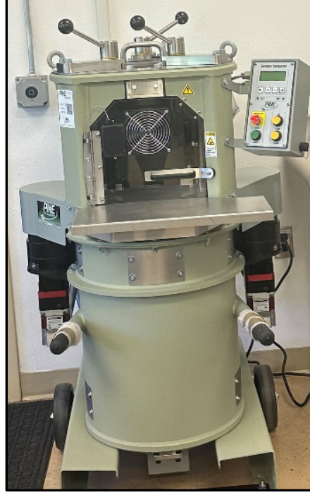
Figure 3.17. Superpave gyratory compactor used in the present study
