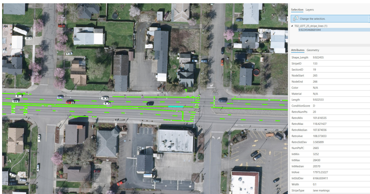
Figure C-0-6. Example output of the csv2gdb.py script showing attributes available in the stripe table.
