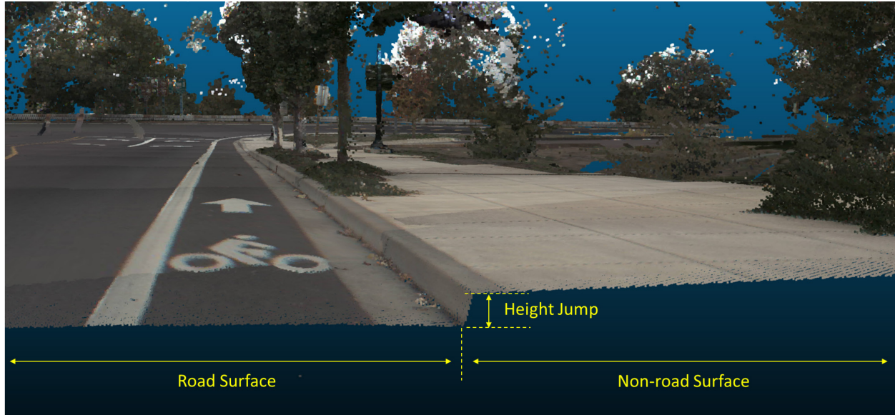
Figure 2-18: Example of the height jump along the curb, serving as a road boundary in point cloud data.
