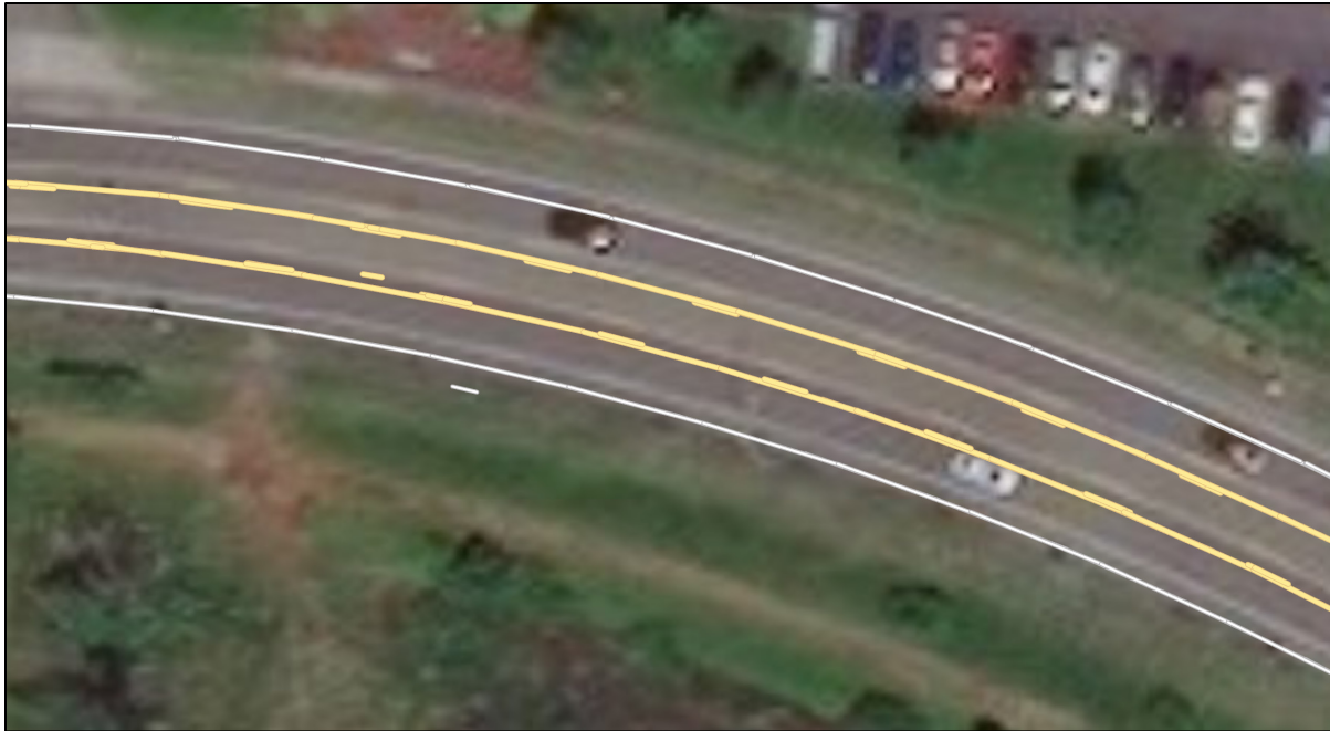
Figure C-0-8. Example output of the stripeEditor.py script showing correct yellow and white stripes with transverse stripes removed.
