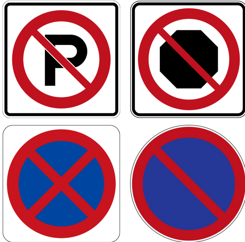
Figure 7-2: Examples of regulatory no parking (left) and no stopping (right) signs that conform to MUTCD (top) and Vienna Convention (bottom) standards.
