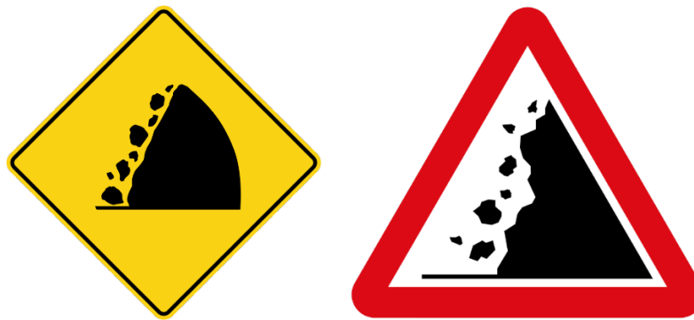
Figure 7-1: Examples of avalanche/rockfall warning signs conforming to MUTCD (left) and Vienna Convention (right) standards.
