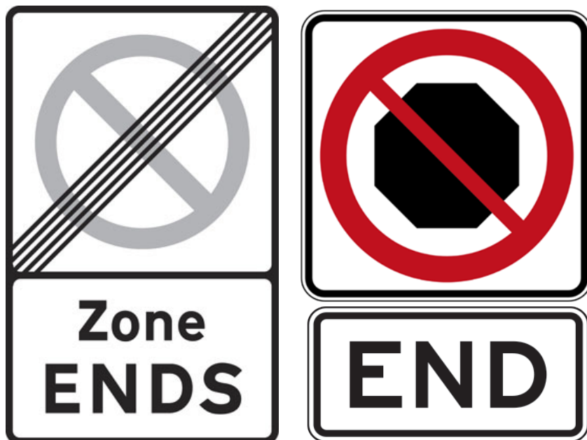
Figure 7-3: Examples of “End of No Stopping” indicative signs that conform to Vienna Convention (left) and MUTCD (right) standards.
