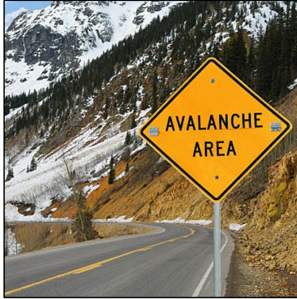
Figure 4-1: Example of a general avalanche-area warning sign intended to prime drivers to be alert for potential avalanche hazards along the roadway ahead.
