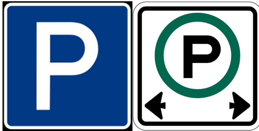
Figure 7-4: Examples of parking permitted indicative signs that conform to Vienna Convention (left) and MUTCD (right) standards.
