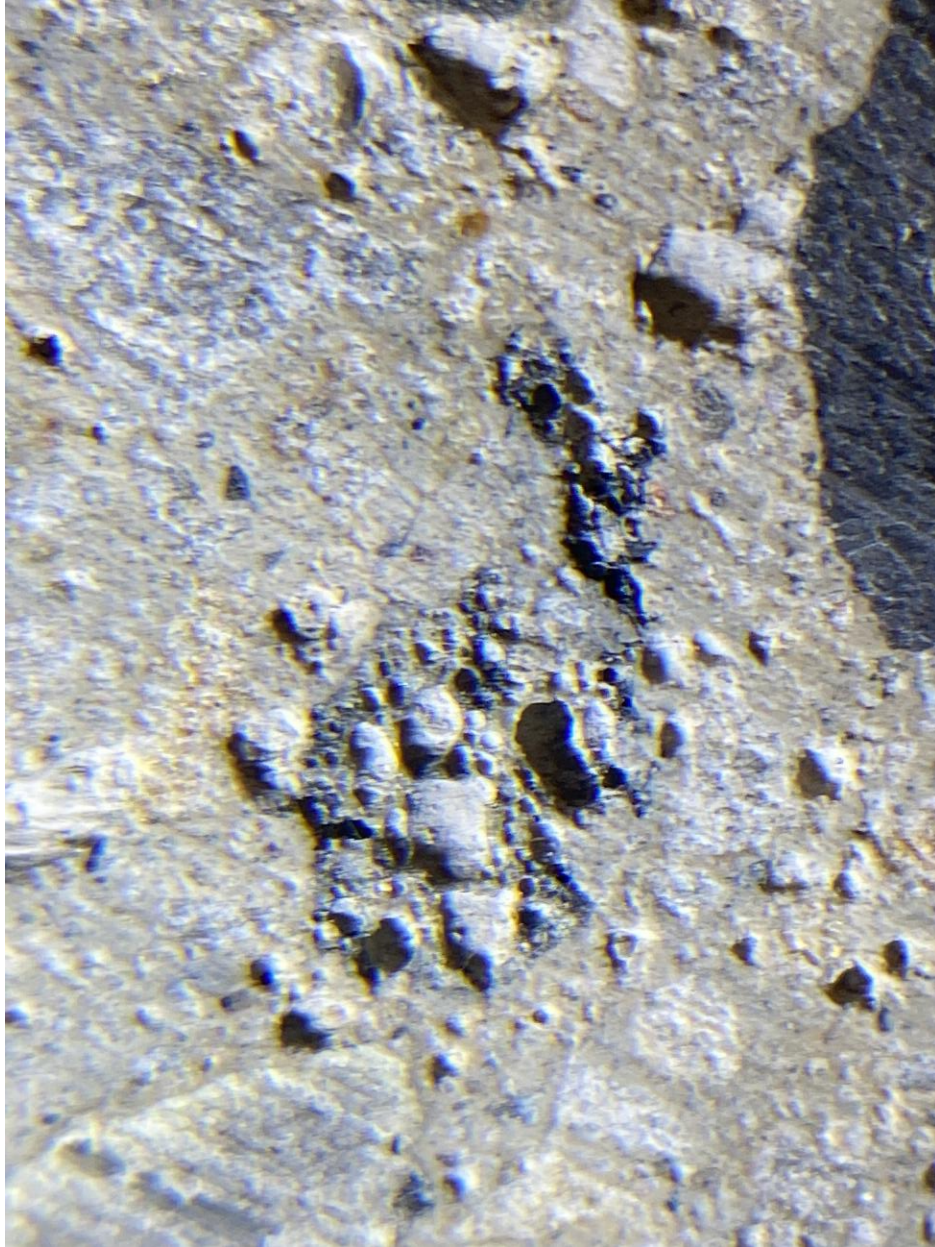
Figure E.4 Aggregate in core 2 of lightweight concrete deck at bridge C-989 (3).
