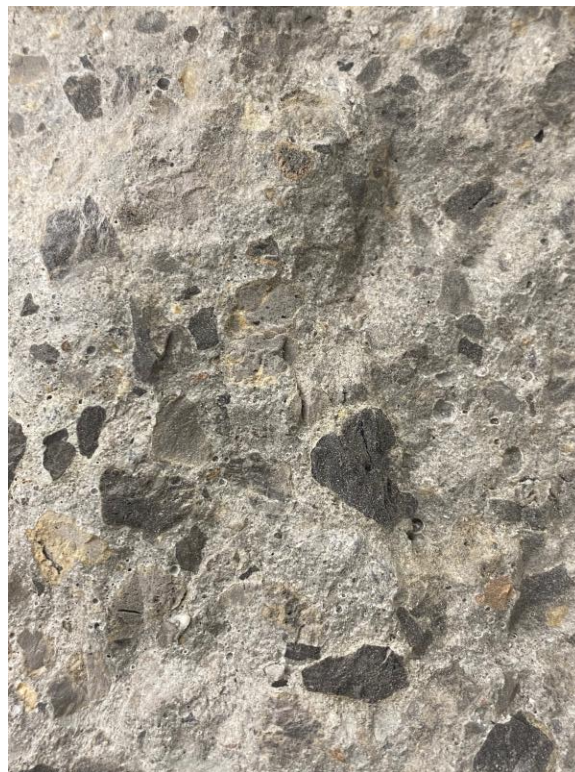
Figure 4.11 Lightweight concrete fracture face.
