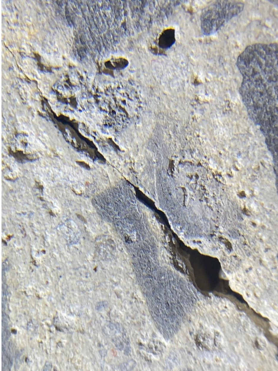
Figure E.6 Aggregate in core 4 of lightweight concrete deck at bridge C-989.
