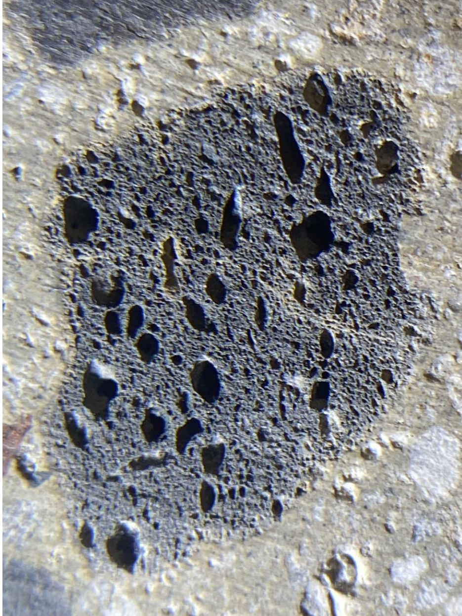
Figure E.7 Aggregate in core 5 of lightweight concrete deck at bridge C-989.
