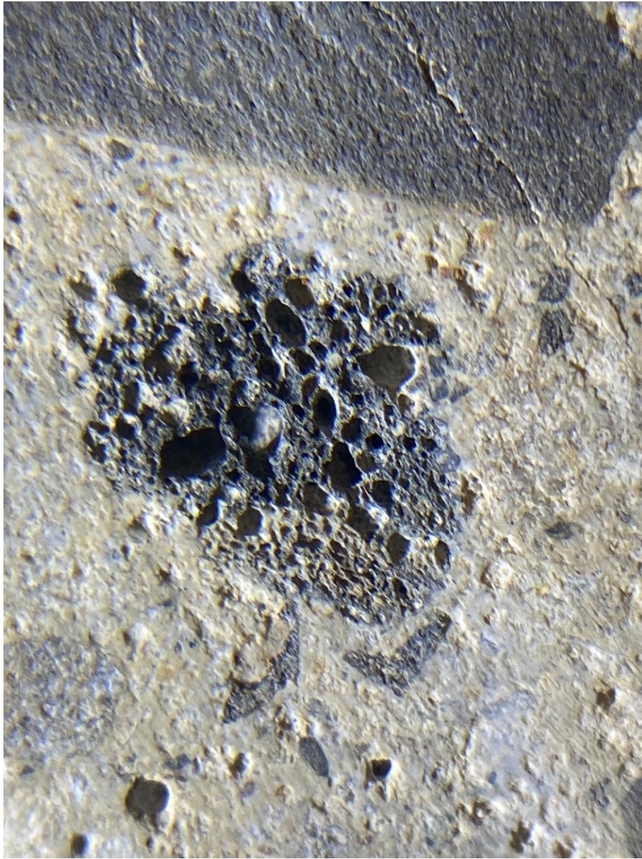
Figure E.1 Aggregate in core 1 of lightweight concrete deck at bridge C-989.
