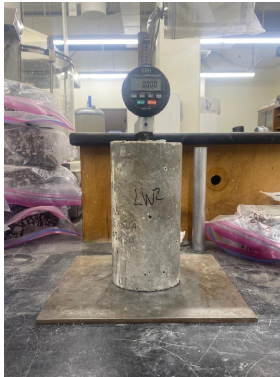
Figure 3.12 Coefficient of thermal expansion testing.
