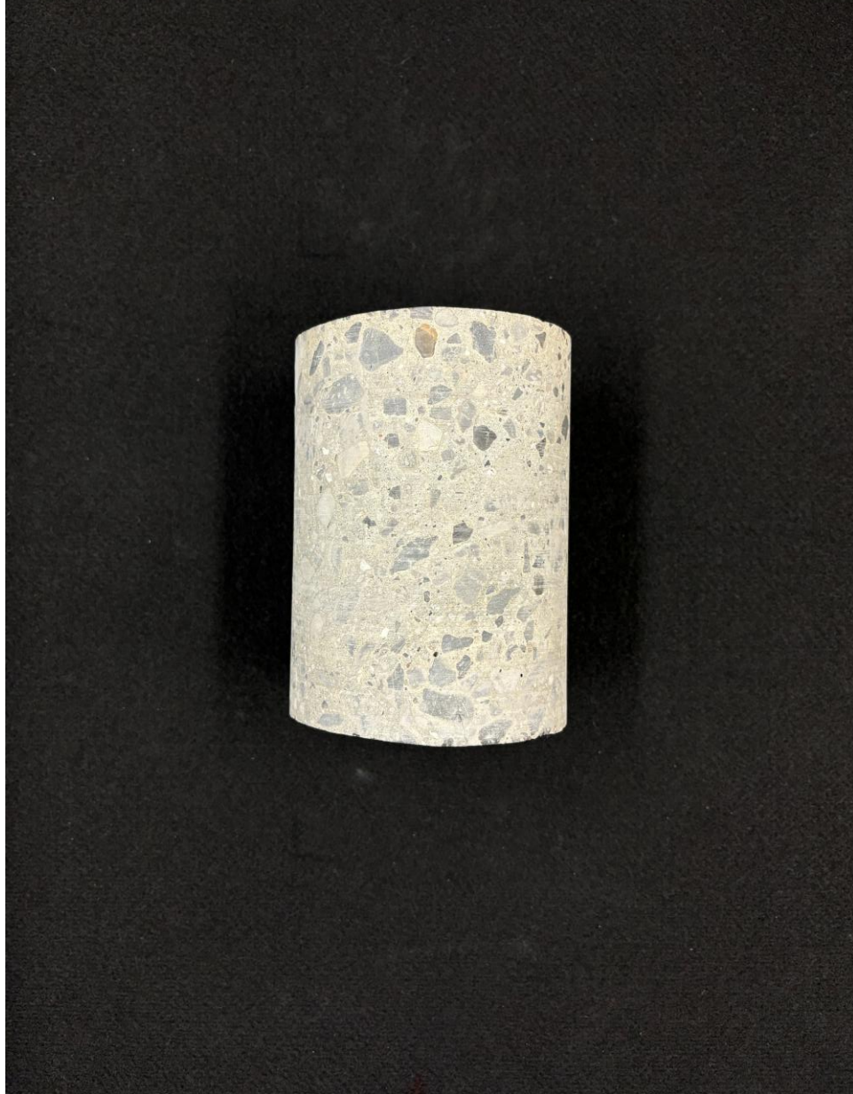
Figure D.14 Core 4 of lightweight concrete deck at bridge F-792.
