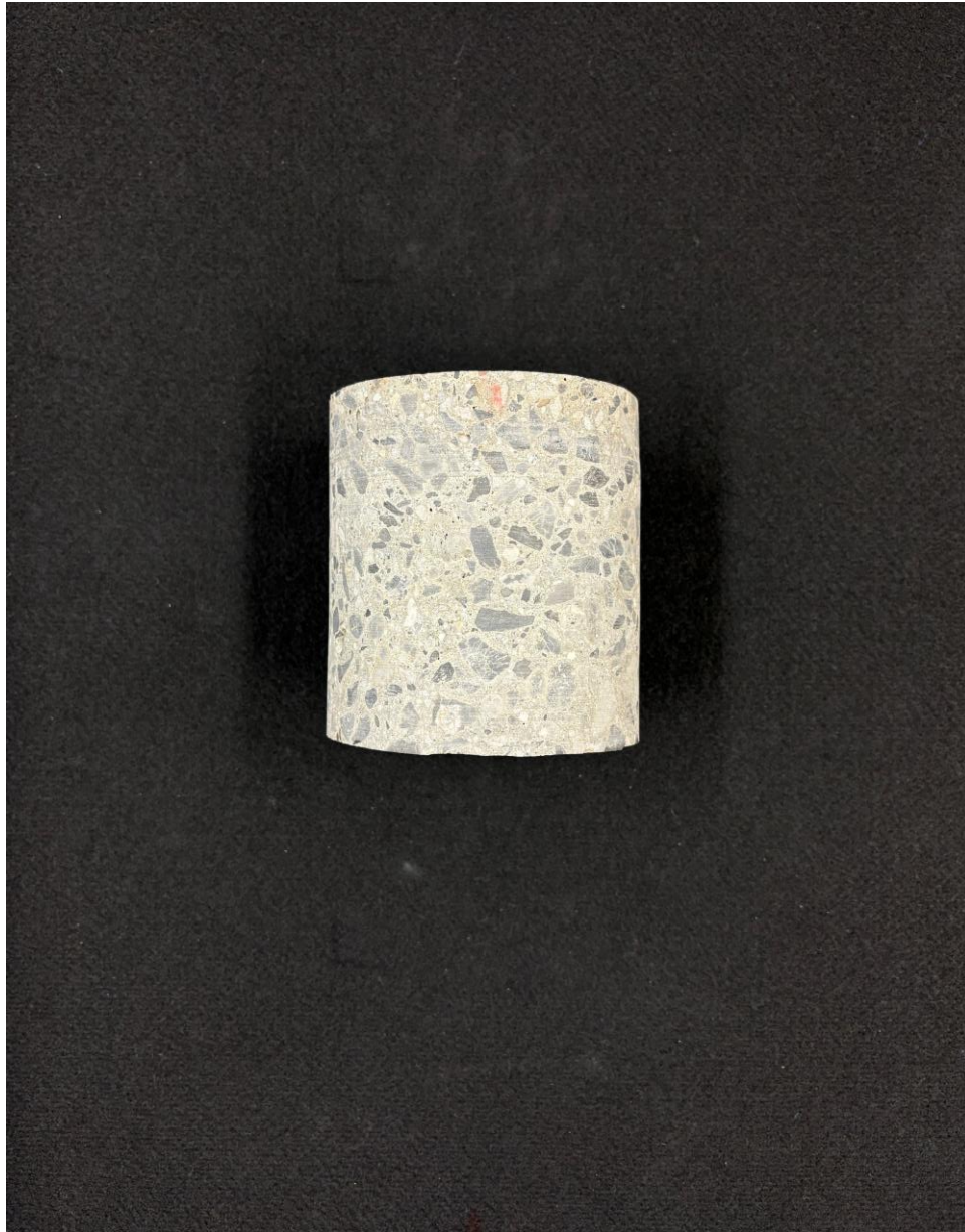
Figure D.11 Core 1 of lightweight concrete deck at bridge F-792.
