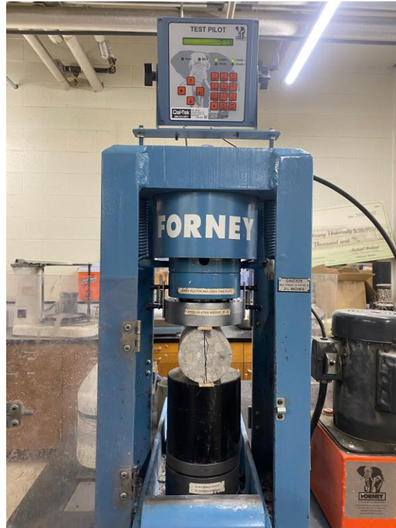
Figure 3.10 Splitting tensile strength testing.
