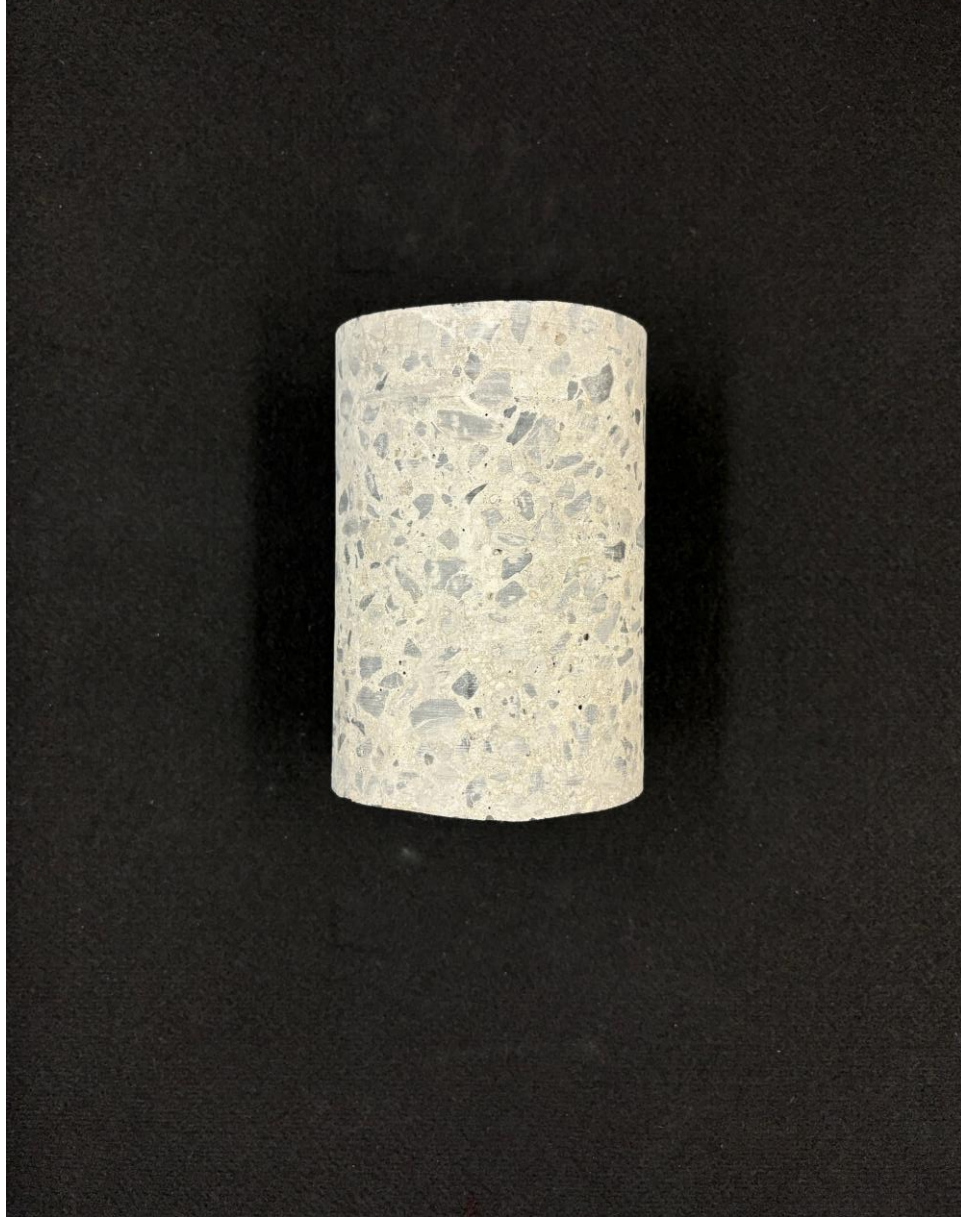
Figure D.3 Core 3 of lightweight concrete deck at bridge C-989.
