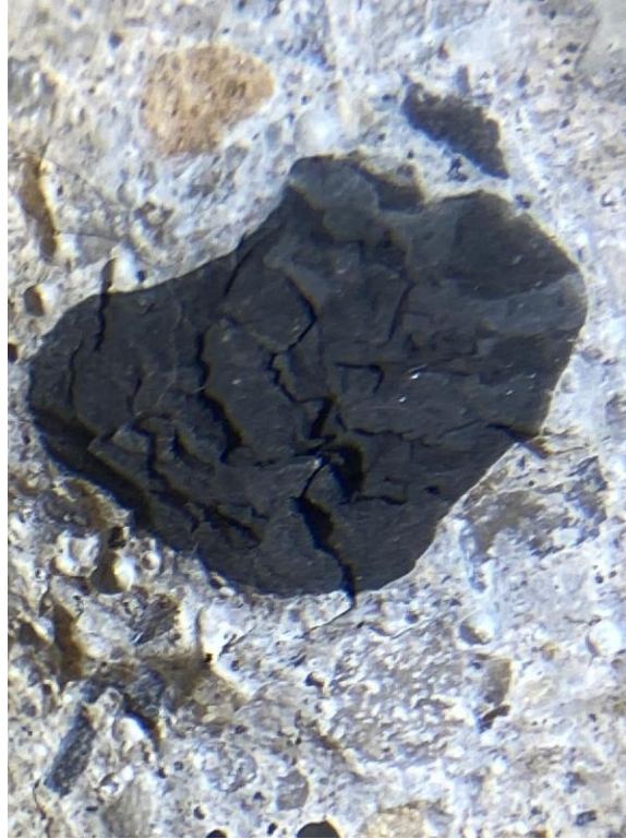
Figure 4.17 Lightweight coarse aggregate fractured during freeze-thaw durability testing.
