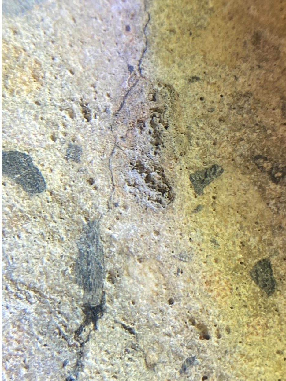
Figure E.10 Aggregate in core 2 of lightweight concrete deck at bridge C-1011 (1).
