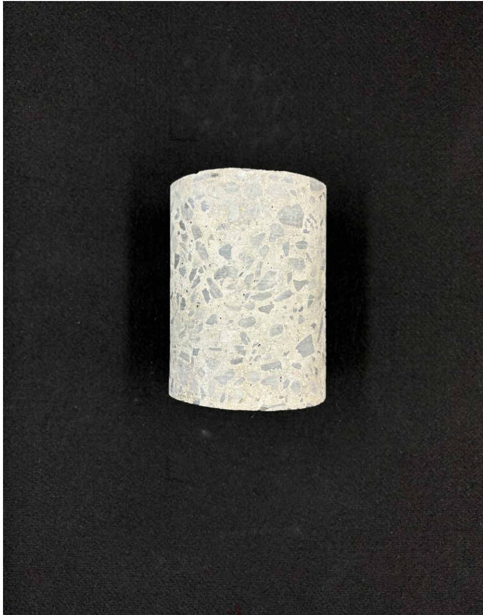
Figure D.5 Core 5 of lightweight concrete deck at bridge C-989.
