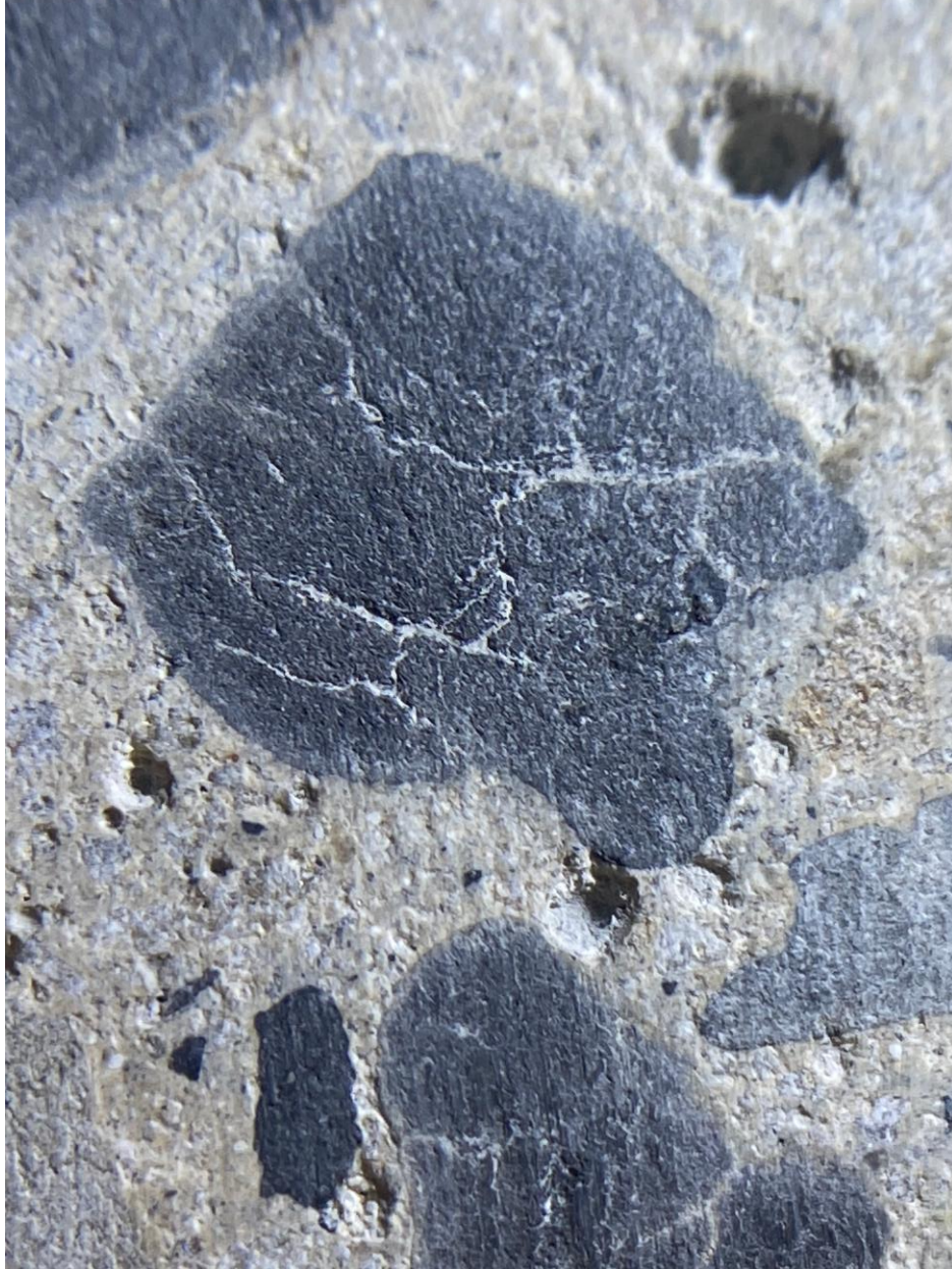
Figure E.14 Aggregate in core 4 of lightweight concrete deck at bridge C-1011.
