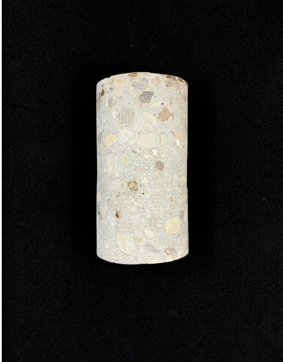
Figure D.18 Core 3 of normal-weight concrete approach slabs at bridge C-989.
