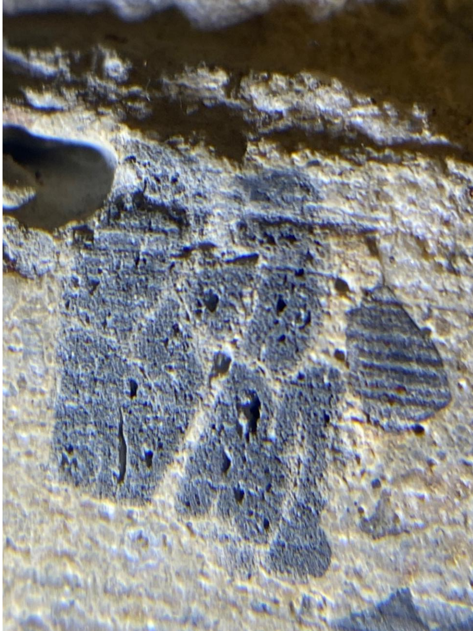
Figure E.13 Aggregate in core 3 of lightweight concrete deck at bridge C-1011 (2).
