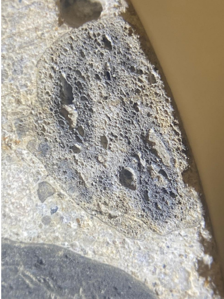
Figure E.2 Aggregate in core 2 of lightweight concrete deck at bridge C-989 (1).
