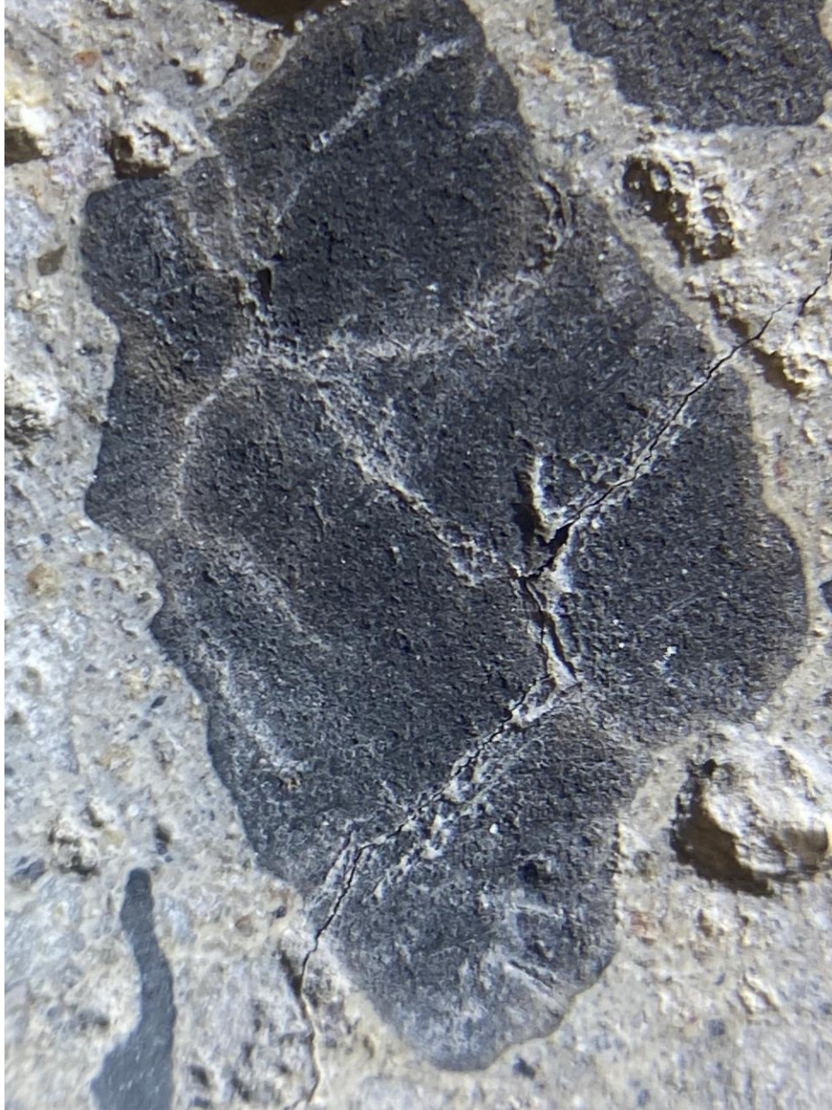
Figure E.5 Aggregate in core 3 of lightweight concrete deck at bridge C-989.
