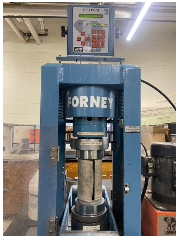
Figure 3.9 Compressive strength testing.
