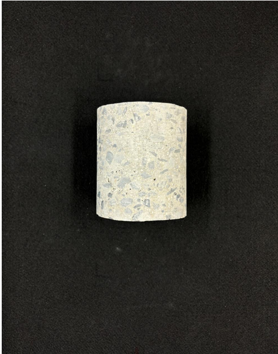
Figure D.4 Core 4 of lightweight concrete deck at bridge C-989.
