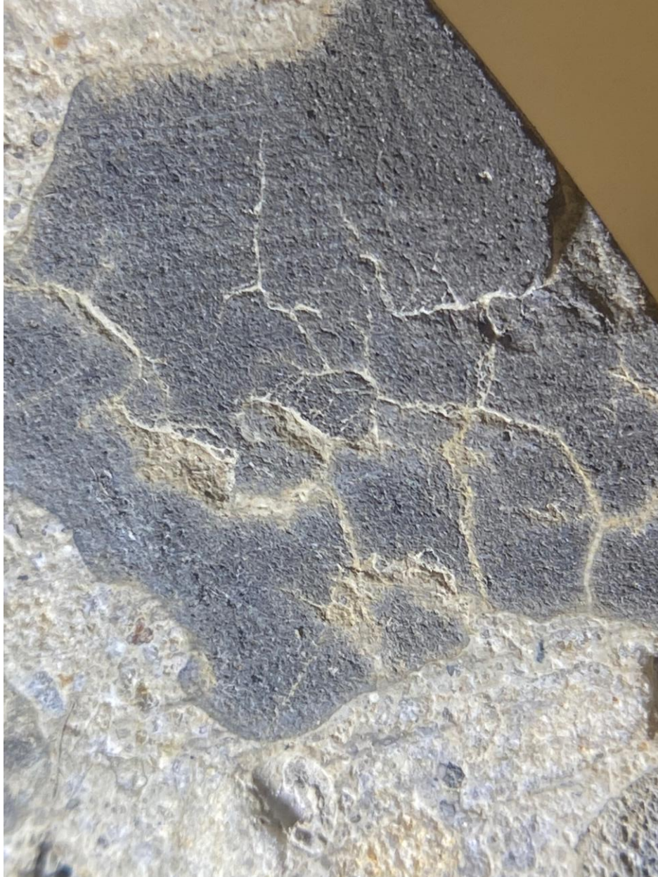
Figure E.3 Aggregate in core 2 of lightweight concrete deck at bridge C-989 (2).
