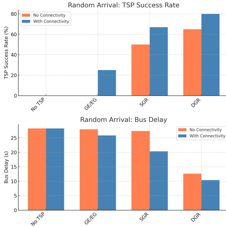
Figure 2: Comparison of TSP Success Rate and Bus Delay Under Random Vehicle Arrivals
