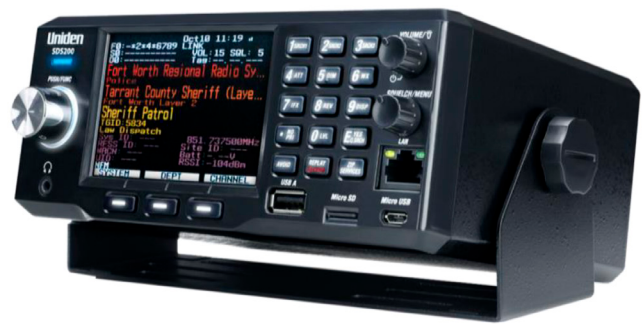
Figure 2.3 The Uniden SDS200 Advanced Digital Scanner, Selected for Widespread Deployment Due to its Integrated LAN Port and IP-Based Remote Control Capabilities (Uniden, n.d.b).
