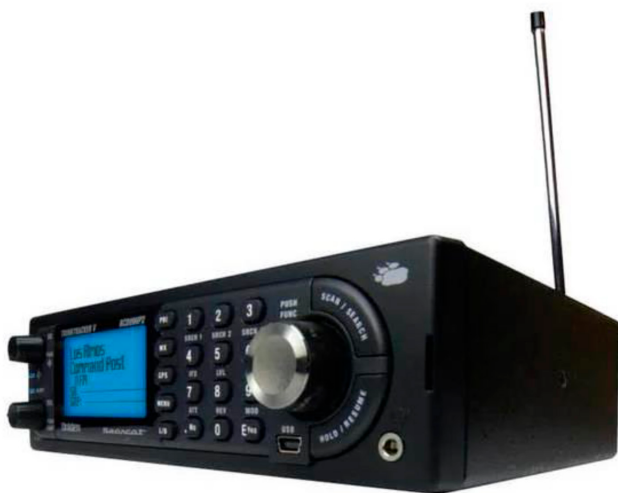
Figure 2.2 The Uniden BCD996P2 Digital Trunking Scanner Used for Initial Prototype Sites and Legacy System Monitoring (Uniden, n.d.a).
