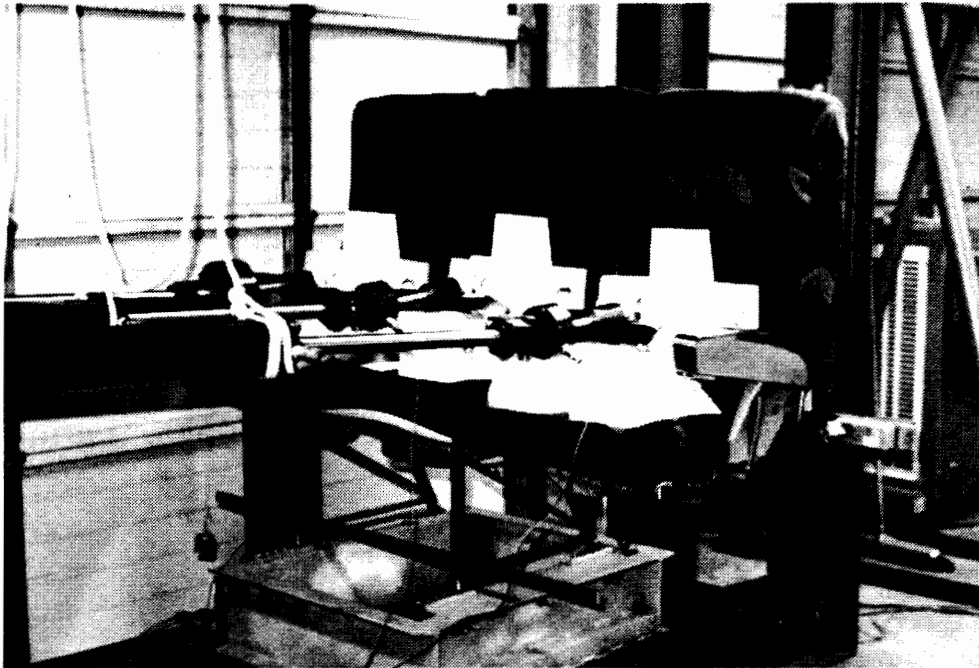
Figure 16. Forward static test arrangement.
