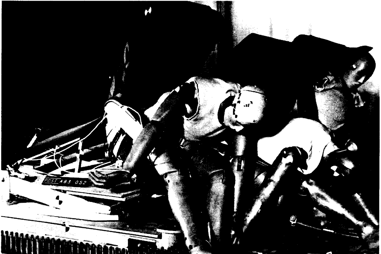
Figure 20. Standard seat after dynamic testing.
