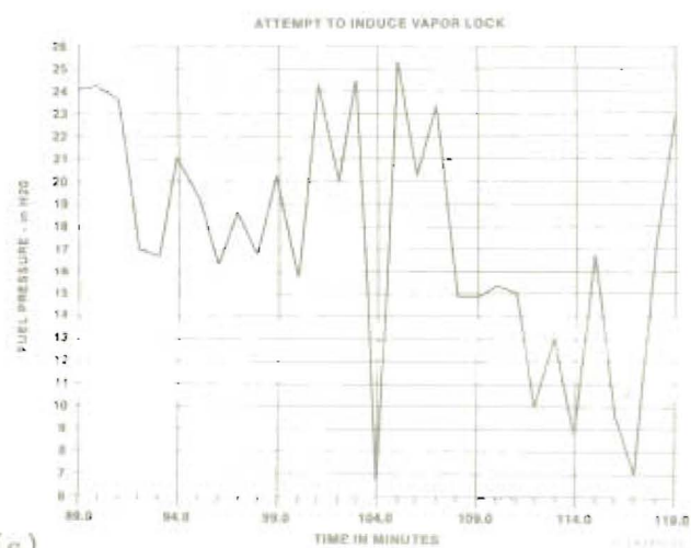
FIGURE 4. FUEL SYSTEM TEMPERATURES, FUEL FLOW AND PRESSURE DURING AN ATTEMPT TO INDUCE VAPOR LOCK WITH AVGAS
