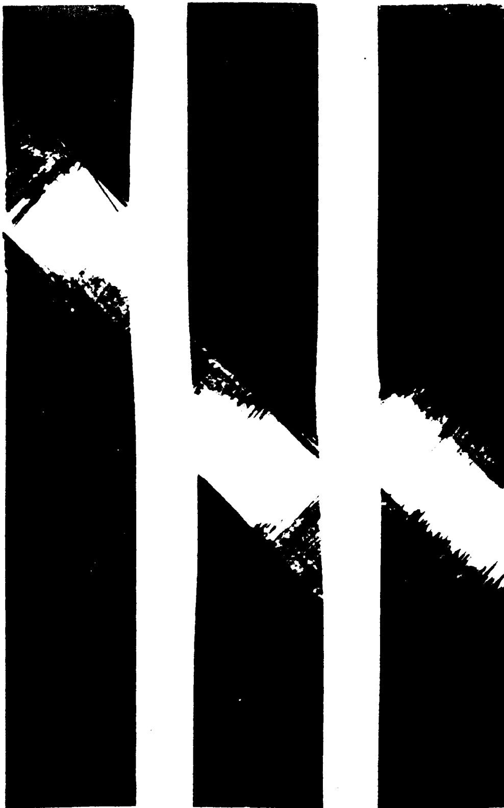
Figure 3.43 Typical Failures of [\pm 45]_s Boron/Epoxy Laminates Subjected to Longitudinal Tension-Tension Fatigue Loading
