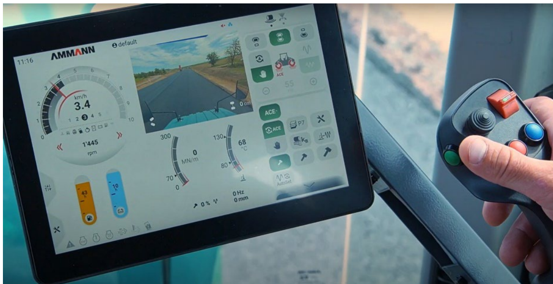
Figure 119. Roller Equipped with IC Technology
