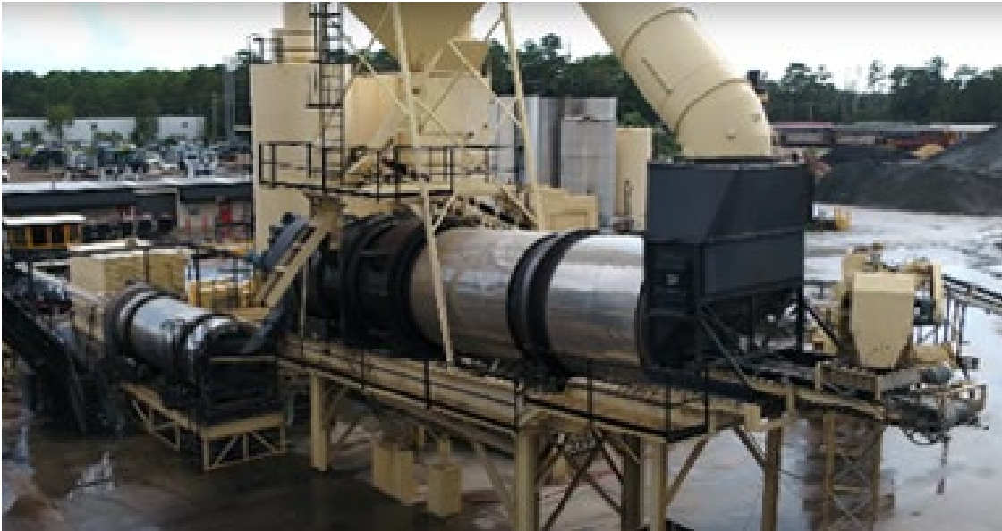
Figure 29. Typical Batch Plant Dryer
