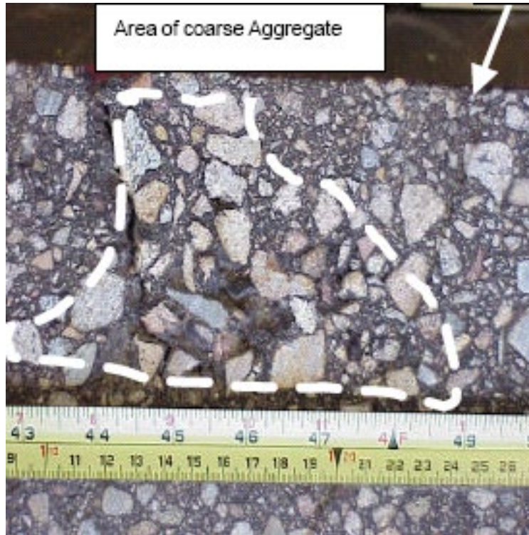
Figure 153. Vertical Segregation (Top Different than Bottom of Cross Section)
