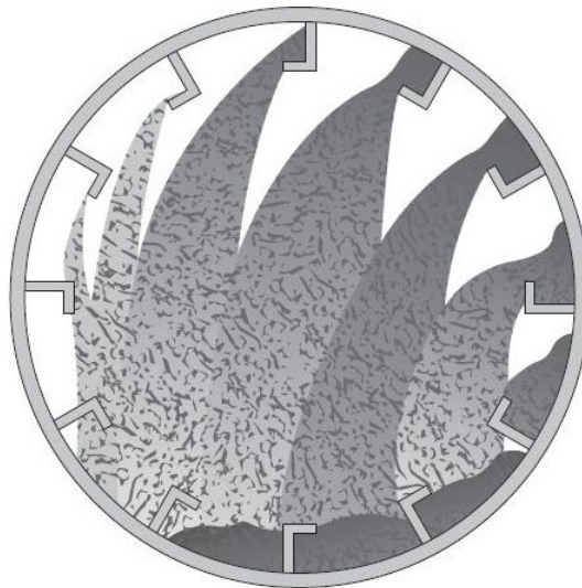
Figure 30. Uniform Veil of Aggregate in Dryer
