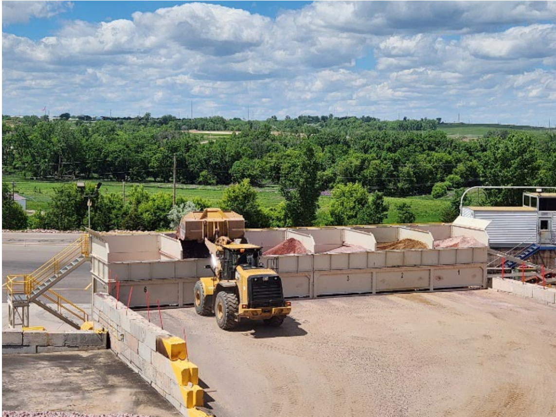
Figure 24. Loading Aggregate Cold-Feed Bins
