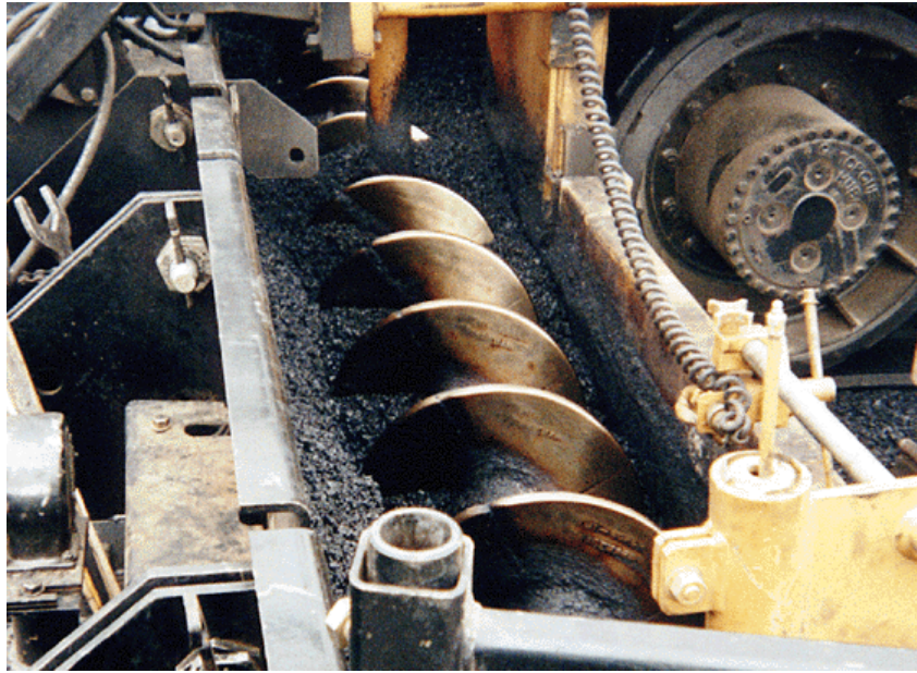
Figure 158. Proper Mix Height in the Auger Box
