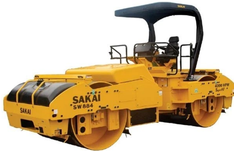
Figure 120. Double-Drum Vibratory Roller Equipped with IC Technology
