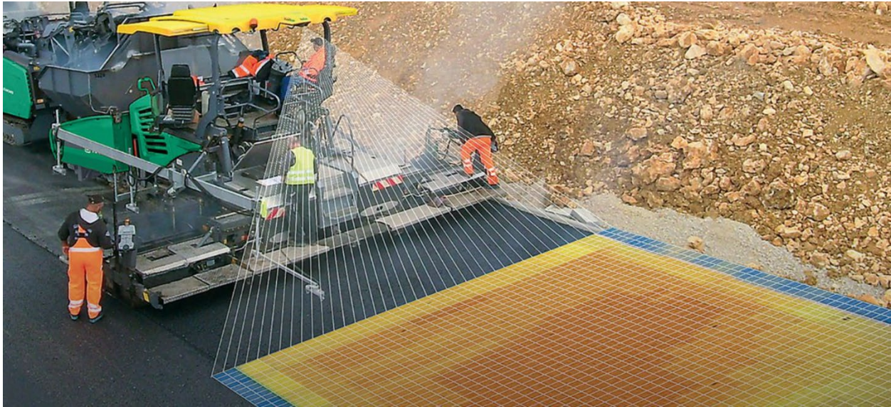
Figure 159. Paver Equipped with an Automated Infrared Scanner
