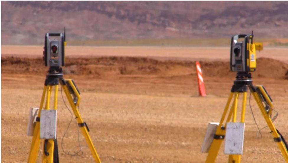
Figure 108. Universal Total Station Tracking Paver
