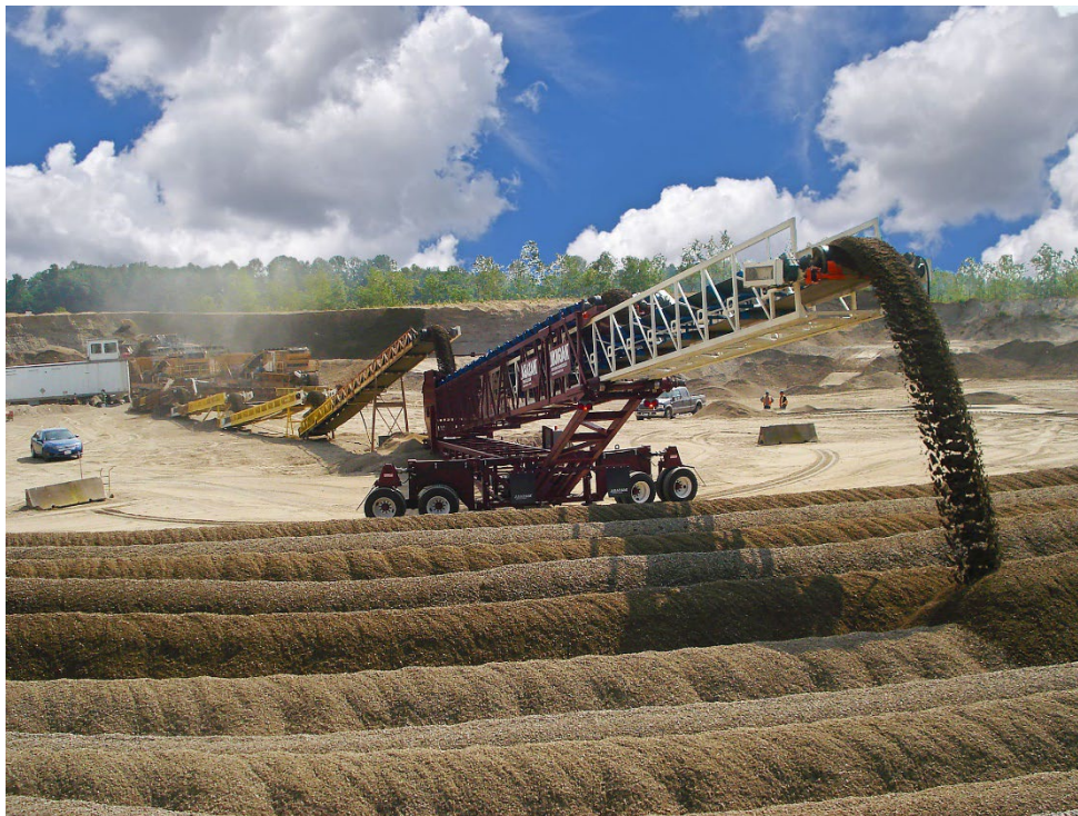
Figure 23. Magnum Telescoping Conveyor Building a Stockpile in Windrows
