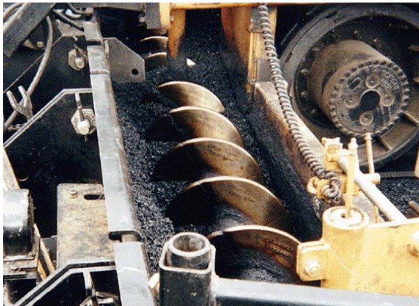
Figure 85. Uniform Head of Material at Axle Height
