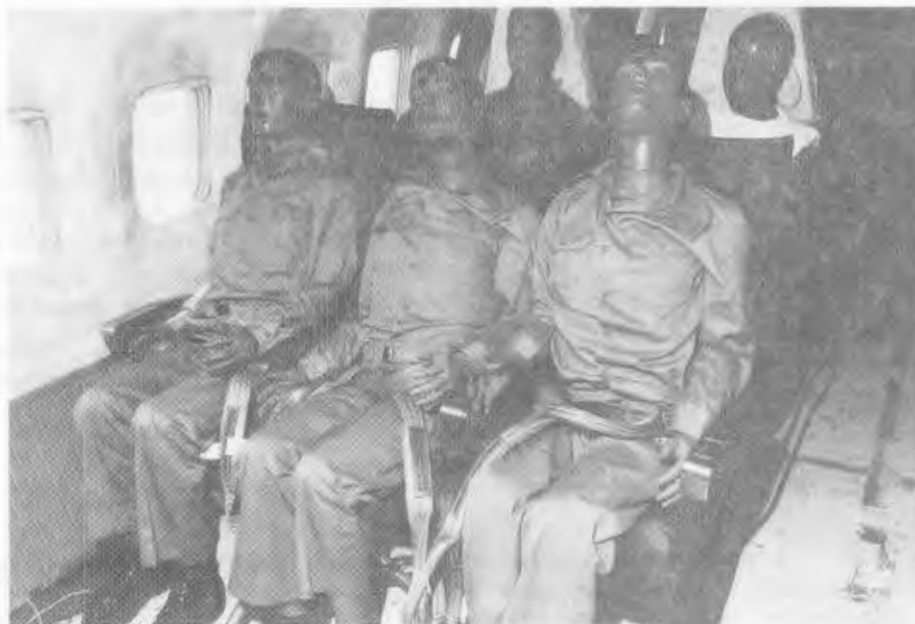
FIGURE 4-A. MEDIUM CLOSE UP PHOTOGRAPH OF DUMMIES IN SIMULA SEATS
