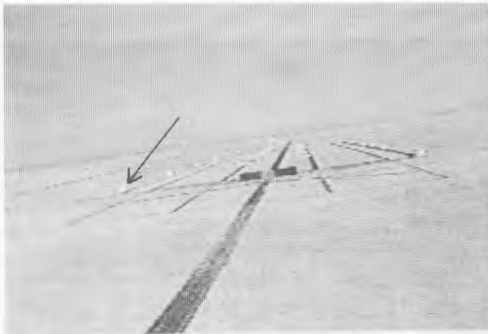
FIGURE 6. NOSE CAMERA COVERAGE SHOWING APPROACH TO IMPACT, CALIBRATION POSTS, AND FLASH BULB SYNCHRONIZATION LIGHTS (ARROW)
