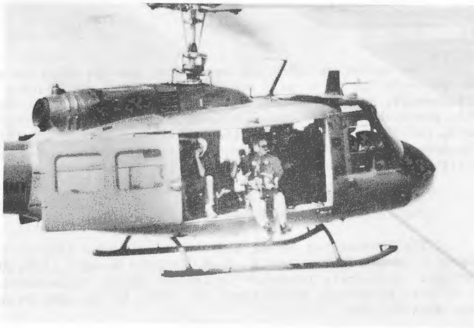
FIGURE 1. ARMY HELICOPTER WITH PHOTOGRAPHER SEATED IN GYRO-CONTROLLED MOUNT
