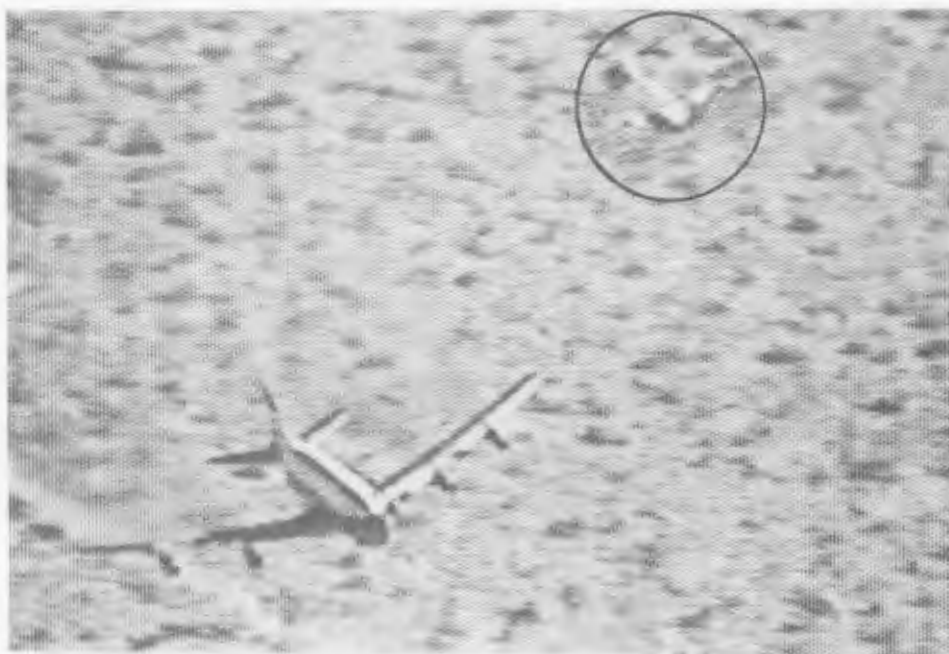
FIGURE 28. CID AIRCRAFT APPROACHING IMPACT AND CHASE PLANE (IN CIRCLE) (VIEW FROM CAST GLANCE)
