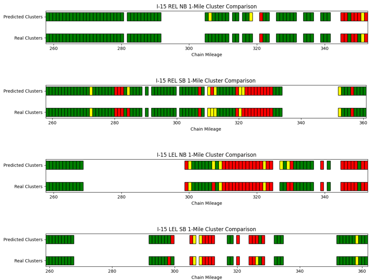
Figure 5-36 Segment Classification for I-15 – Predicted vs. Field-Based Retroreflectivity
