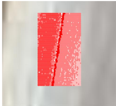
Figure 3-2 Filtering to Identify Lane Markings
