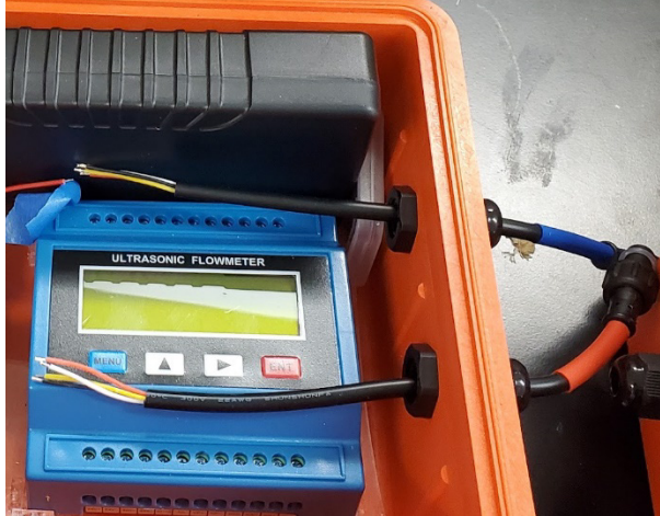
Figure 7.24 Pelican case with waterproof connector cables, battery, and flow meter.
