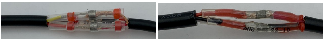
Figure 7.19 Waterproof connector cable and transducer cable wires with solder seal connectors prior to heating (left) and after heating (right). Note directions indicate putting on and heating each connector individually, not all together as shown on the left.
