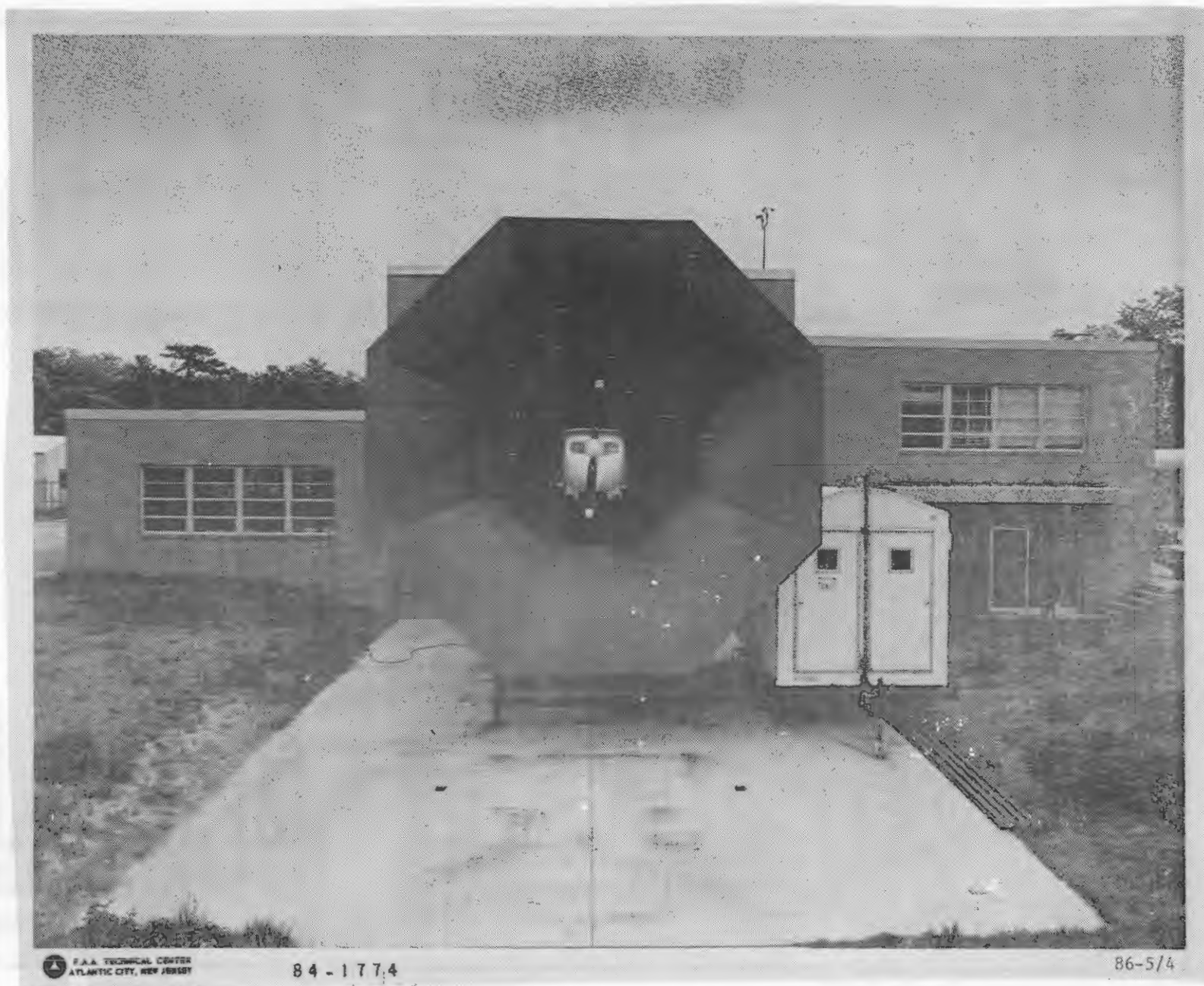
FIGURE 3. CESSNA 210C AIRPLANE WITHIN AVIATION FLOW FACILITY TEST SECTION
