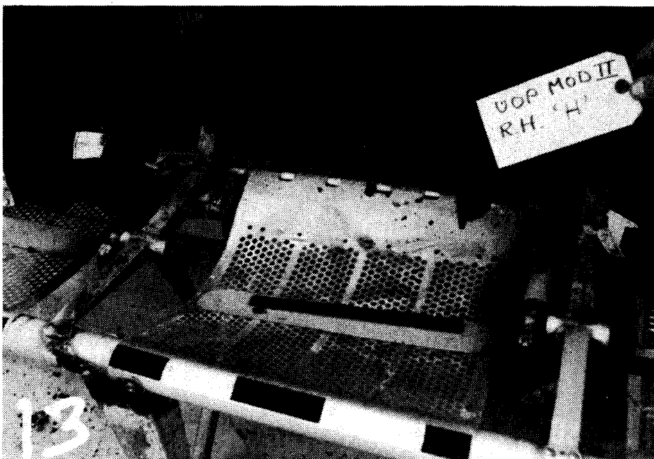
Figure 55. Seat pan deformation of seat H/R.
