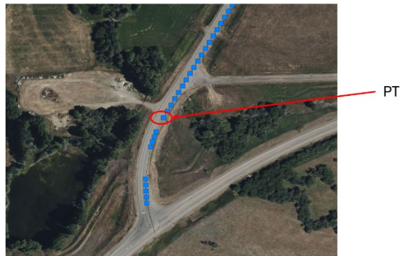
Figure 7. Point of tangency (PT) identified between the curve element and tangent element based on the difference in bearing of successive elements
