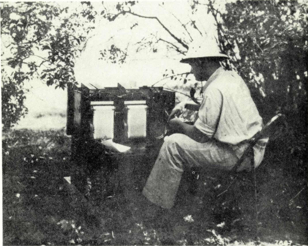
Graphic Recorders Employed in Field Studies of Vehicle Passing Practices and Random Truck Performance.
