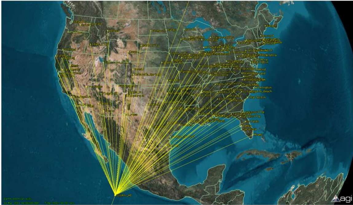
Figure 4b. Spaceborne GPS RX Occultation Scenario – Mainbeam of Array Antenna is Pointed 26.2° Below the Satellite Local Horizontal Towards the Earth Limb
