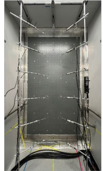
Probes configured to measure the inner two columns. Outer two columns measured in another run.
