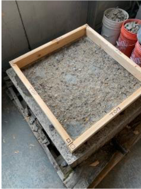
Figure 3-6. Slab in saturated surface dry (SSD) condition and frame for pouring in place.
