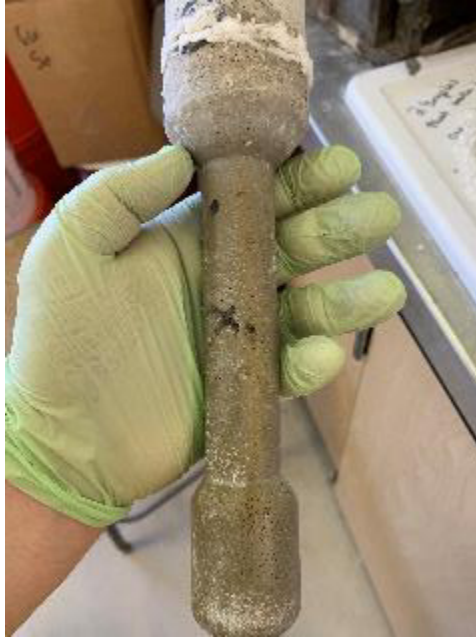
Figure 4-28. Corrosion precipitate and staining on PrCSA2 sample
