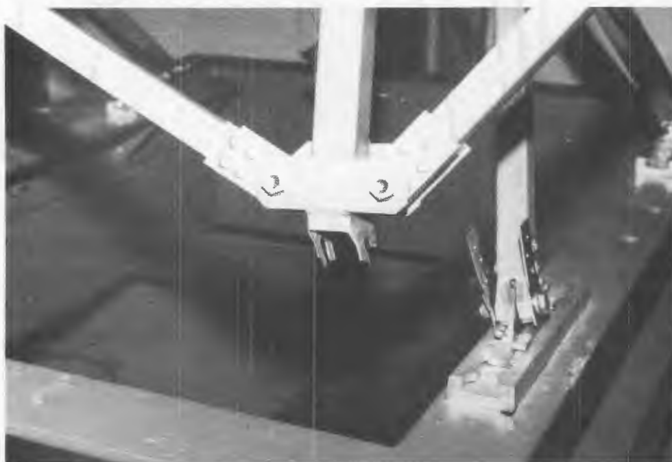
Figure 66. Failure point on Weber MOD I seat (Lateral Test).
