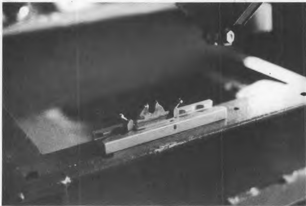
Figure 82. Failure point on the Weber MOD II seat (Lateral Test).
