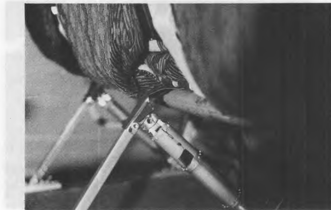
Figure 106. Posttest failed window-side fitting on UOP MOD I seat (Forward Static Test).
