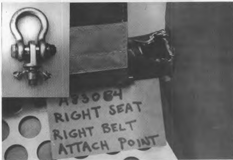
Figure 156. Lap belt anchorage failure point and anchor (inset) of Weberlite MOD seat (Dynamic Test).
