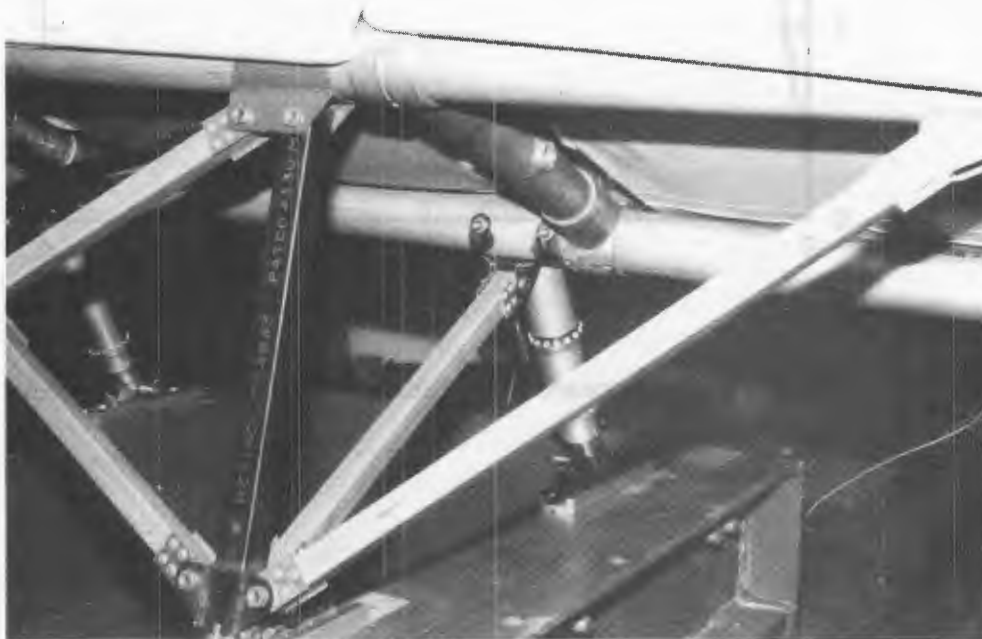
Figure 168. Posttest damage to front tube bracket of Weber aft-facing MOD seat (Forward Static Test).
