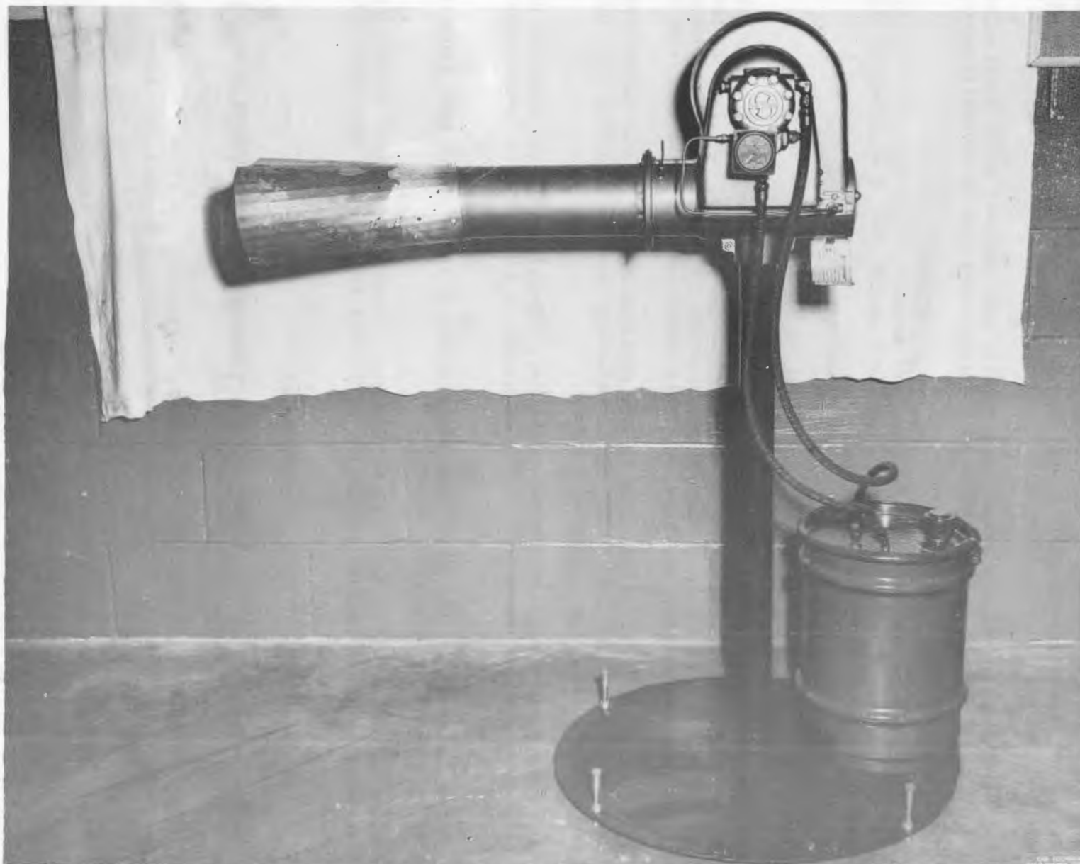
FIGURE 1. PHOTOGRAPH OF 2-GALLON/HOUR KEROSENE BURNER
