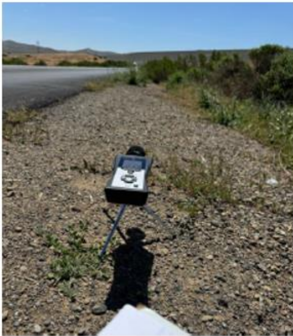
Figure 3. A) PCE sound level meter. B) Gossen MavoMaster light meter. Illuminance Range: 0.001 lx – 199,900 lx. Sampling Rate: 2 measurements per second.
