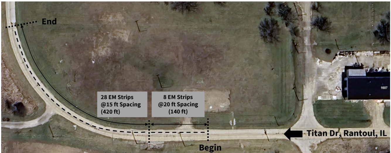
Figure 4. Diagram. Horizontal curve test section (560 ft) on Titan Drive (westbound), Rantoul, Illinois.
