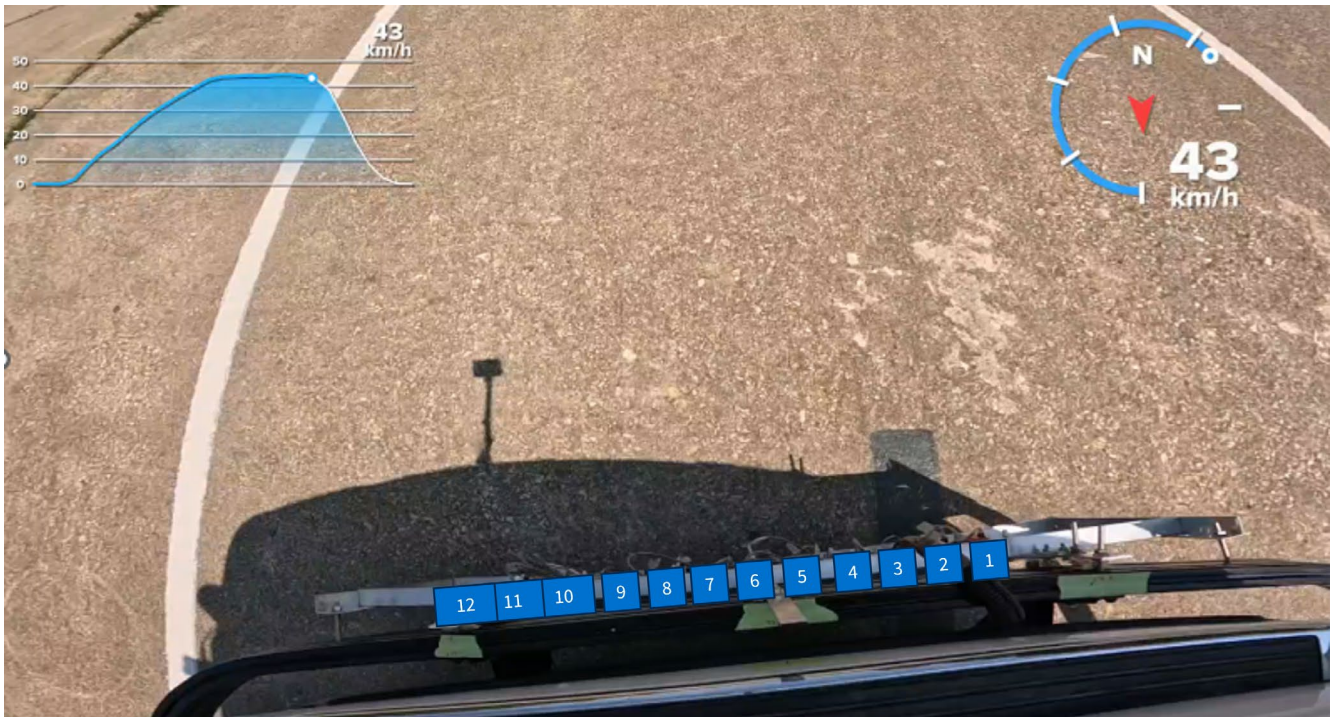
Figure 26. Photo. GPS-camera image when the test vehicle was over the longitudinal strip #4.
