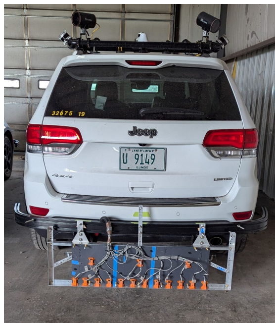
Figure 9. Photo. Magnetometer sensor array setup on the rear bumper of the test vehicle.
