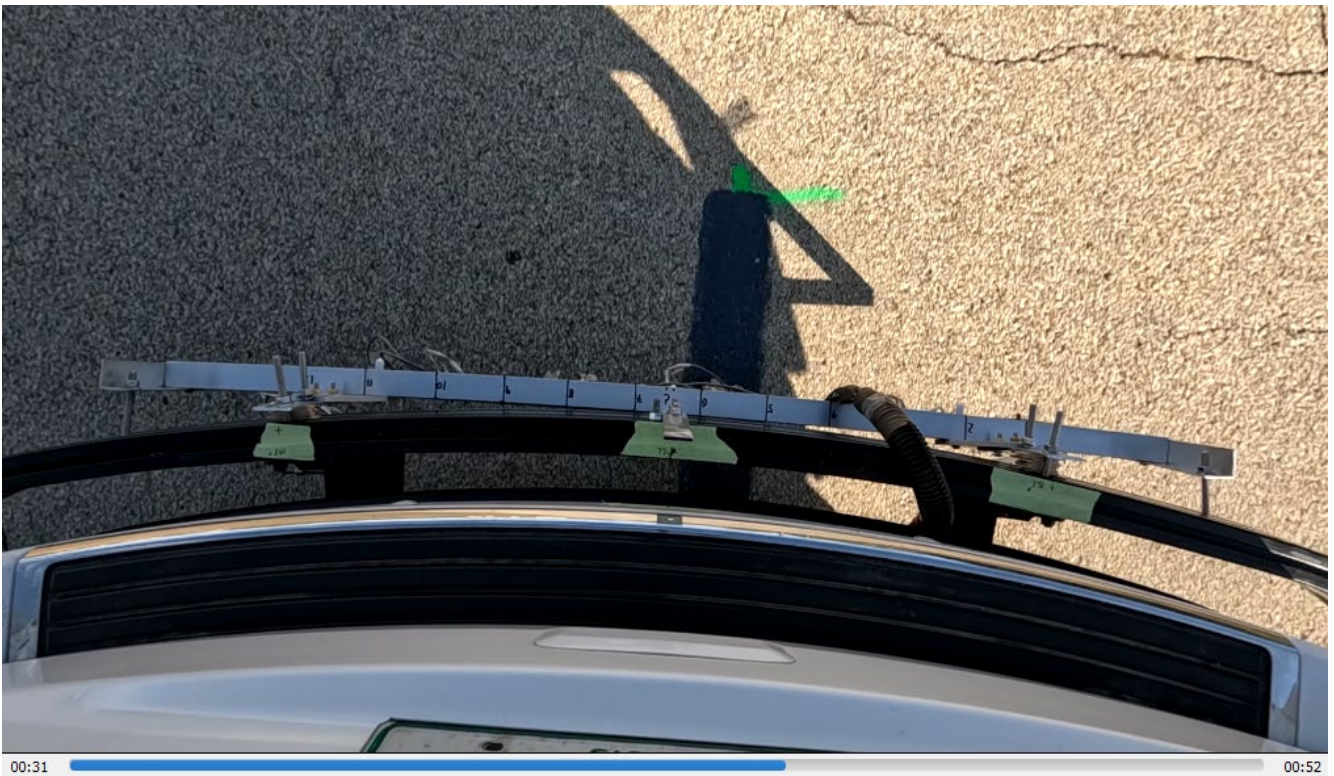
Figure 155. Photo. Referenced photo for longitudinal strip #11 (Case #17).
