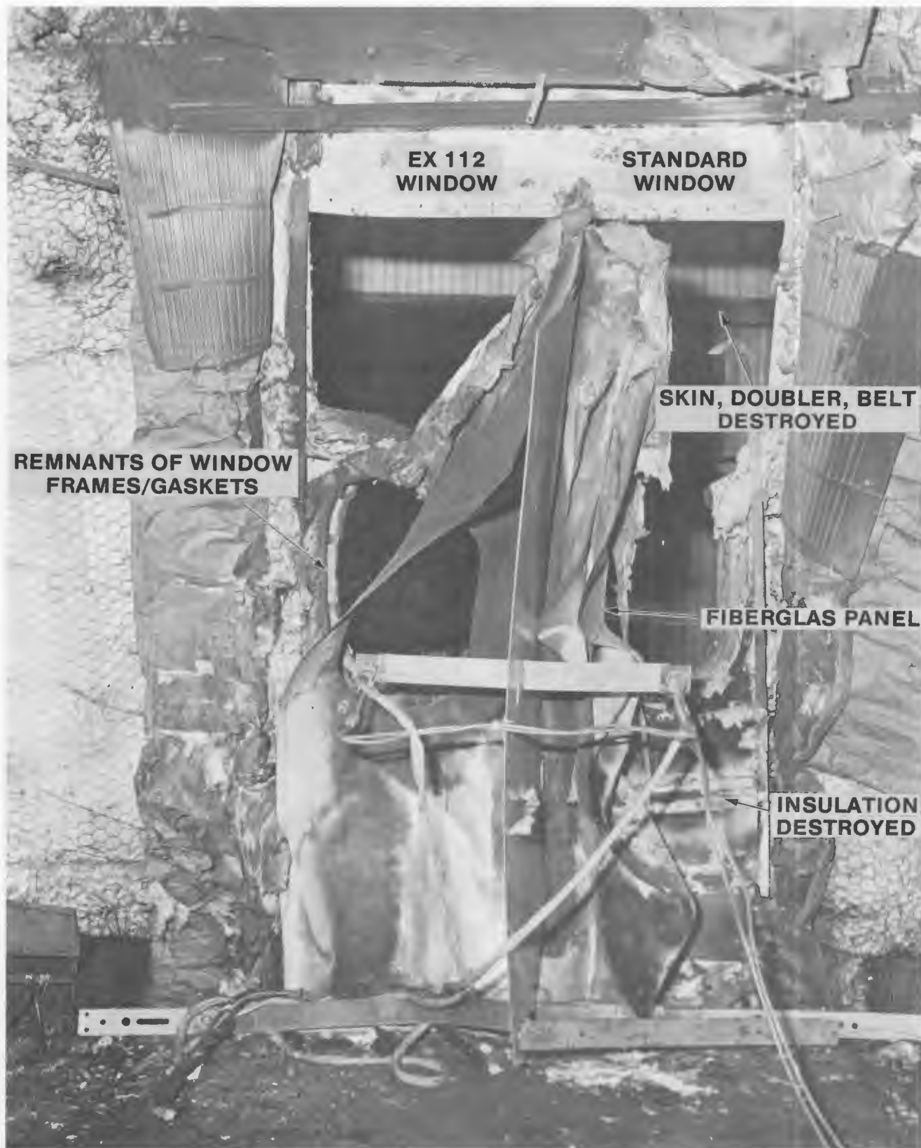
FIGURE 24. FIRE DAMAGE TO THE STANDARD (ACRYLIC) AND IMPROVED (EXIT 112) WINDOWS (TEST 2)
