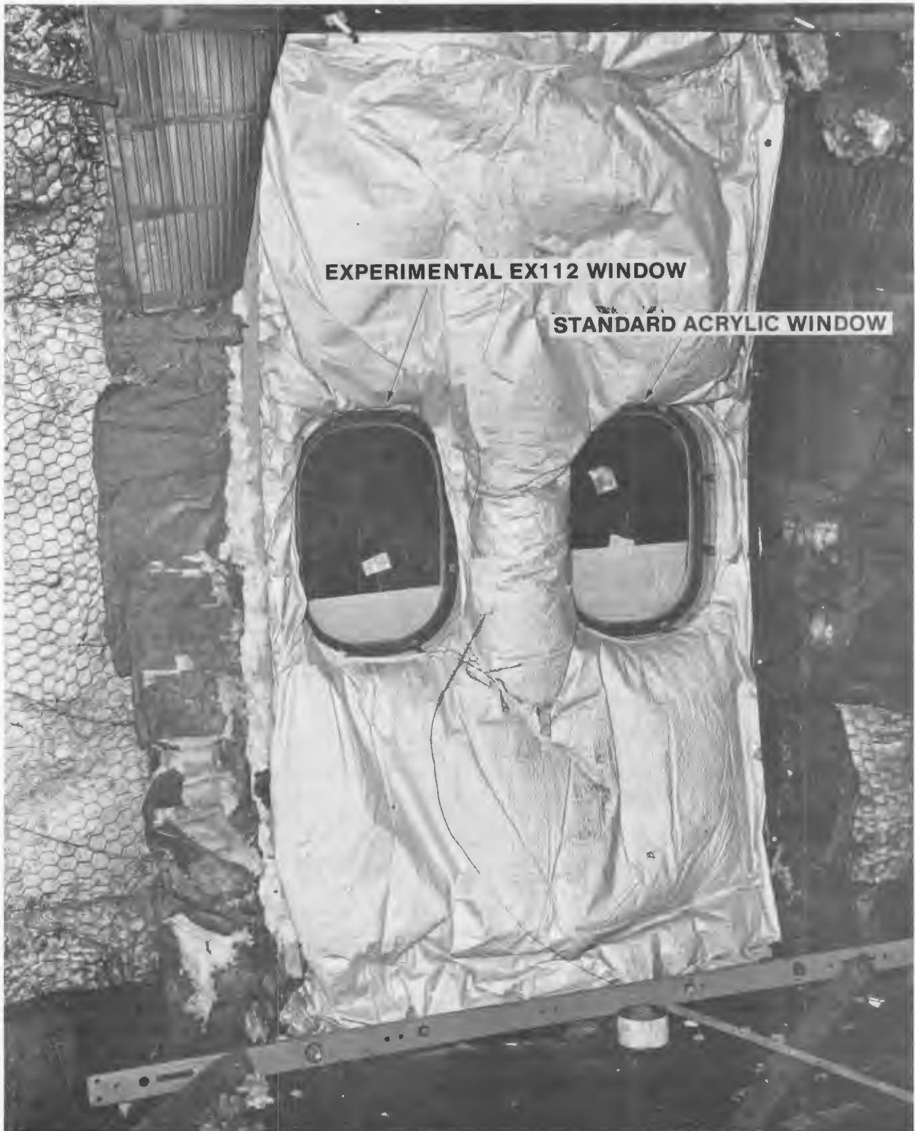
FIGURE 19. STANDARD GLASS FIBER BATT INSULATION INSTALLED IN THE DC-10 WINDOW TEST SEGMENT (TEST 2)
