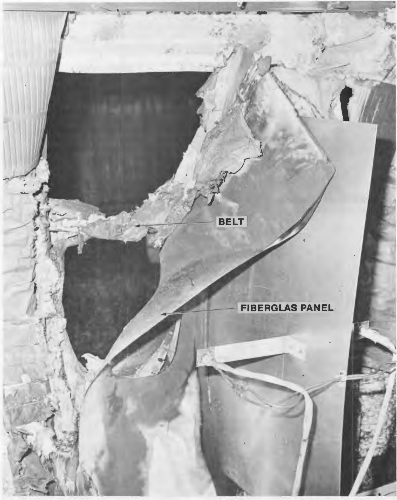
FIGURE 25. CLOSE-UP VIEW OF THE FIRE DAMAGE TO THE IMPROVED (EX 112) WINDOW SYSTEM (TEST 2)
