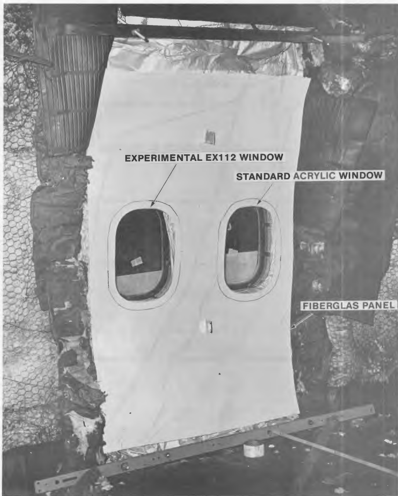
FIGURE 20. FIBERGLASS PANEL IN PLACE OVER THE INSULATION BATT (TEST 2)
