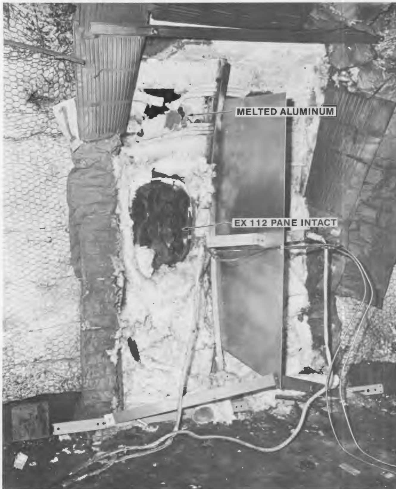
FIGURE 8. FIRE DAMAGE TO THE THERMALLY IMPROVED DC-10 WINDOW SYSTEM SHOWING THE FAIL-SAFE (EX 112) PANE IN PLACE (TEST 1)
