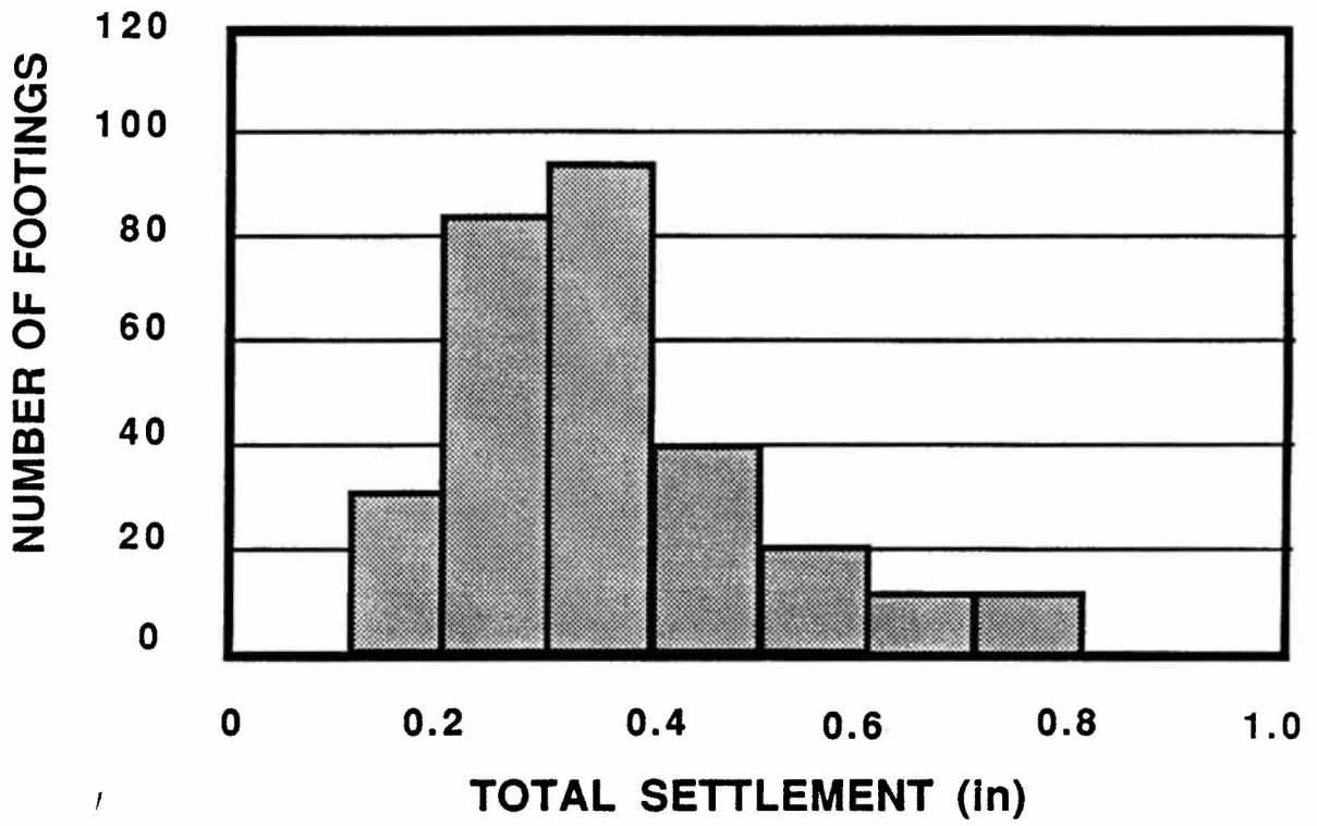
Figure 21. Observed footing settlements.
