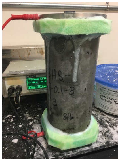
Figure 3. Grout cylinder undergoing bulk resistivity test.
