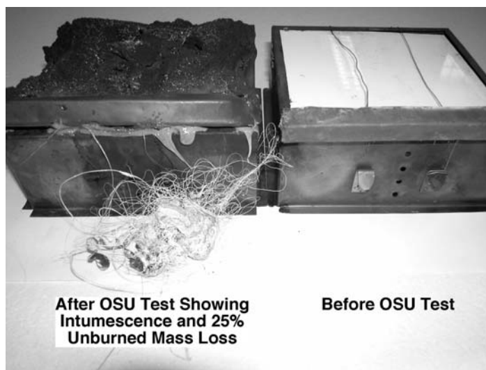
Figure 7. White Polyestercarbonate Before and After 14 CFR Part 25 Testing for HR in the OSU
