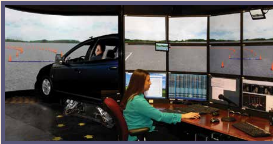
A researcher in the control room monitors testing of the motion base, while a test subject operates FHWA's highway driving simulator.
