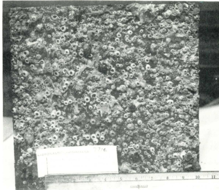
FIGURE 9a - A TYPICAL FOULED PANEL: After immersion at Miami Marine Research, Inc. for three months
