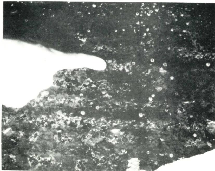
b. CLOSEUP OF RUN 1; CLEANED PATH AND SOME BARE METAL AT 13.8 MPa (2,000 psi); 0.61 m/s (2 ft/s).
