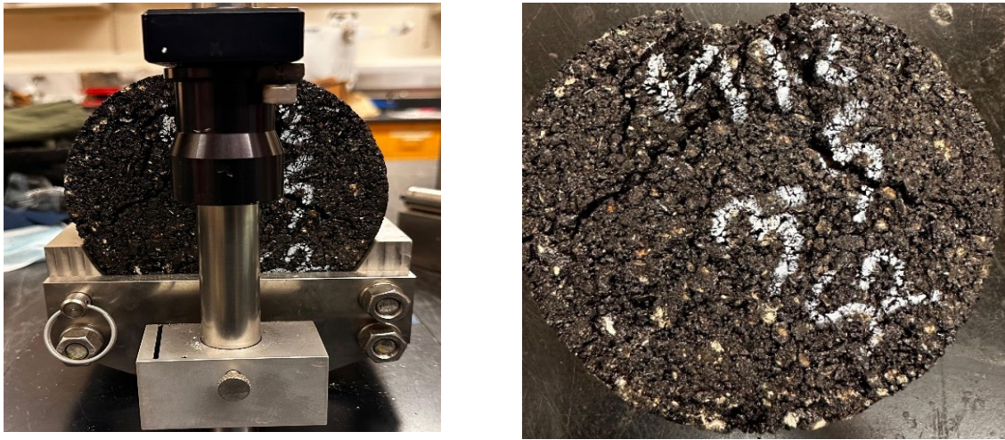
FIGURE 2.80 Ideal-RT test set up
