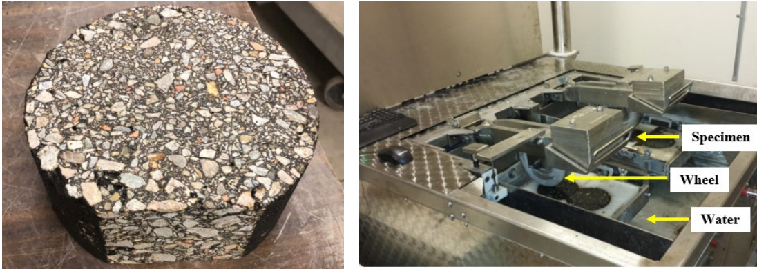
(a) HWTT Prepared Specimen
