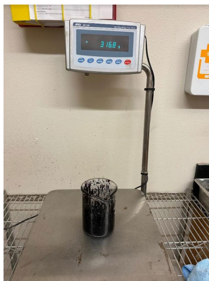
FIGURE 3.4: Weight of breaker, stirrer rod, and emulsion after heating phase
