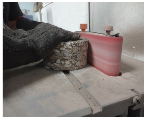
(b) Sand Grinding Field Core's Peripheral Side
