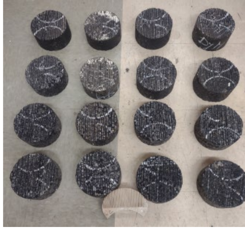
FIGURE 5.40: Prepared controlled notched/grooved specimens (used as bottom layer)
