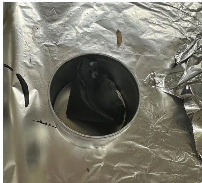
FIGURE 3.5: Residual Asphalt Removed from Filter
