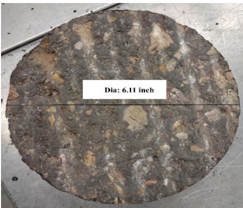
(a) 6.11-Inch Dia Field Core
