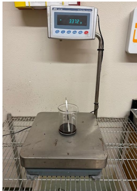
FIGURE 3.2: Weight of beaker, stirrer rod, and emulsion before heating phase
