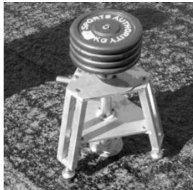
FIGURE 2.19: University of Texas at El Paso (UTEP) in-situ pull-off test (Hakimzadeh, 2015)
