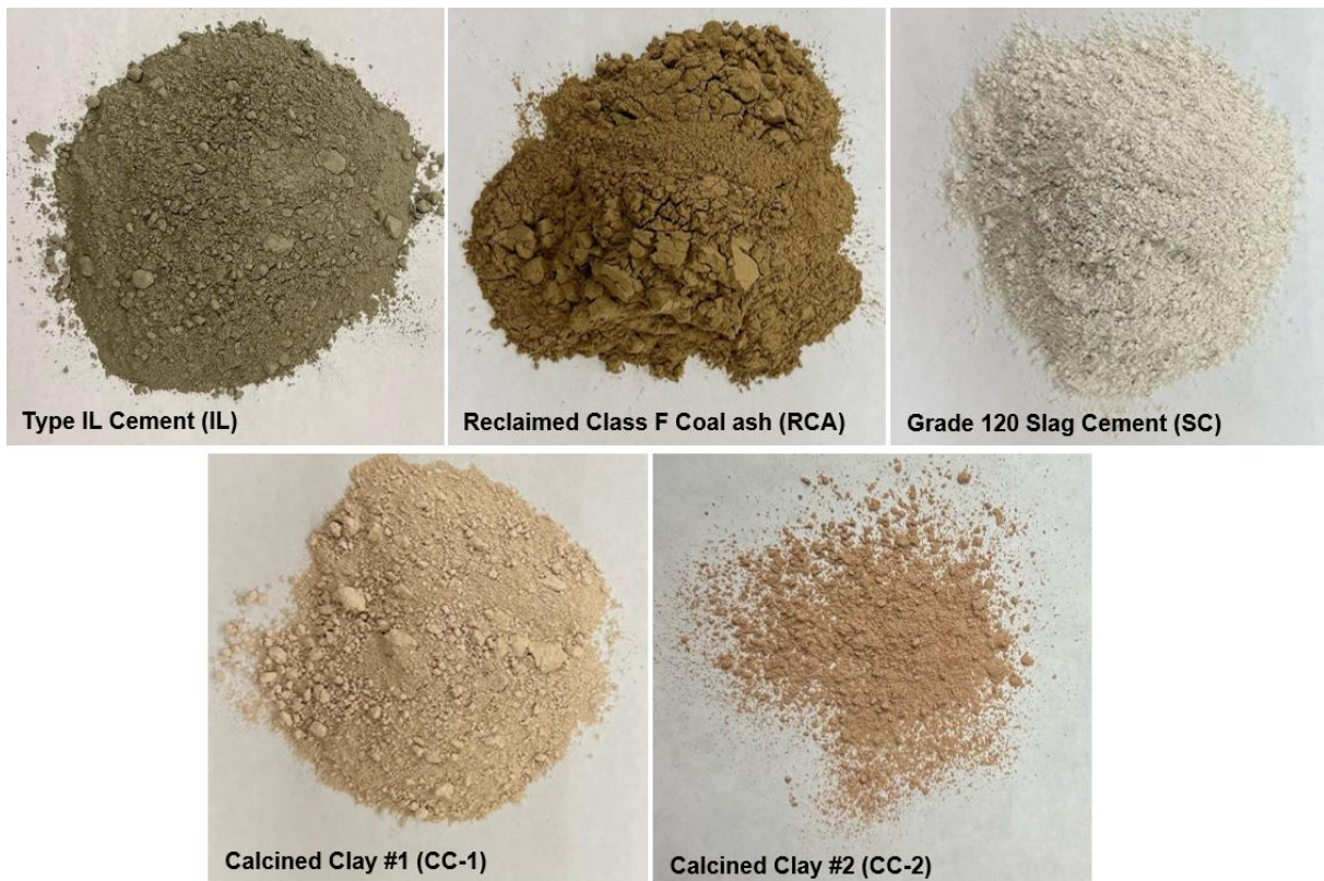
Figure 2. Cement and Supplementary Cementitious Materials Considered in this Study
