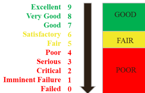
Figure 3. Example of Overall Condition Rating Scale
