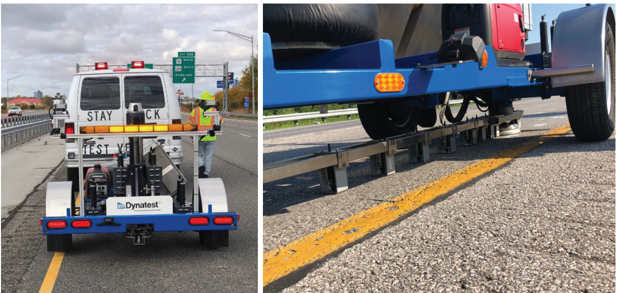
Figure 1.1 INDOT FWD Device (a) View from Behind Device and (b) View of Underneath Device (October 2022).
