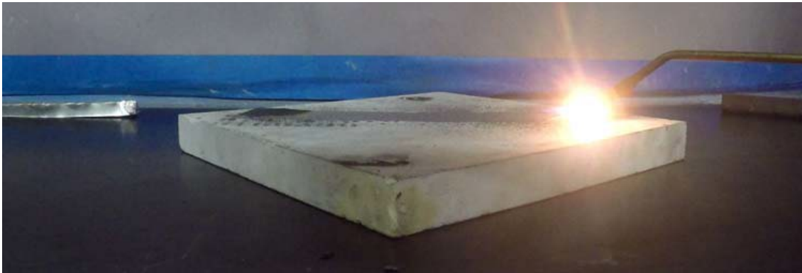
Figure A2-13 Ta-2.5W exposed to butane and propane-oxygen torch flames-no ignition
