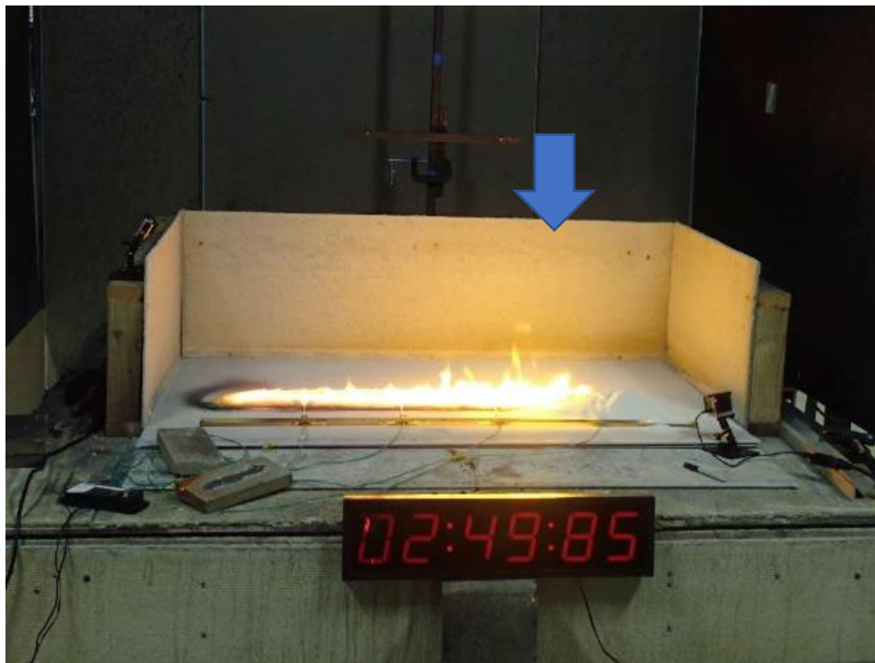
Figure A3-4 Response of -40 mesh titanium sponge to application of Class D agent
