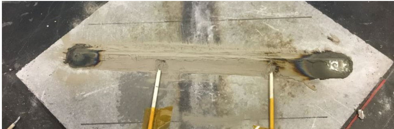
Figure A2-10 Nickel powder did not ignite from butane or propane oxygen torch flames
