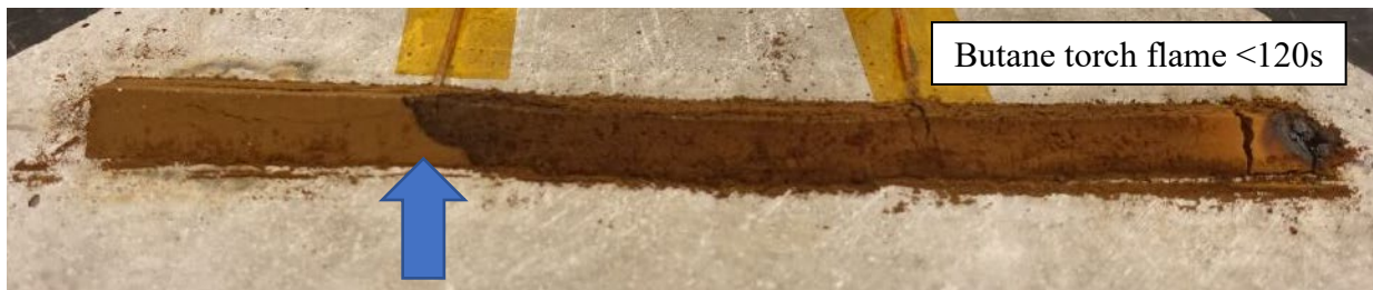
Figure A2-6 Smoldering steel process dust. The blue arrow indicates the smoldering front
