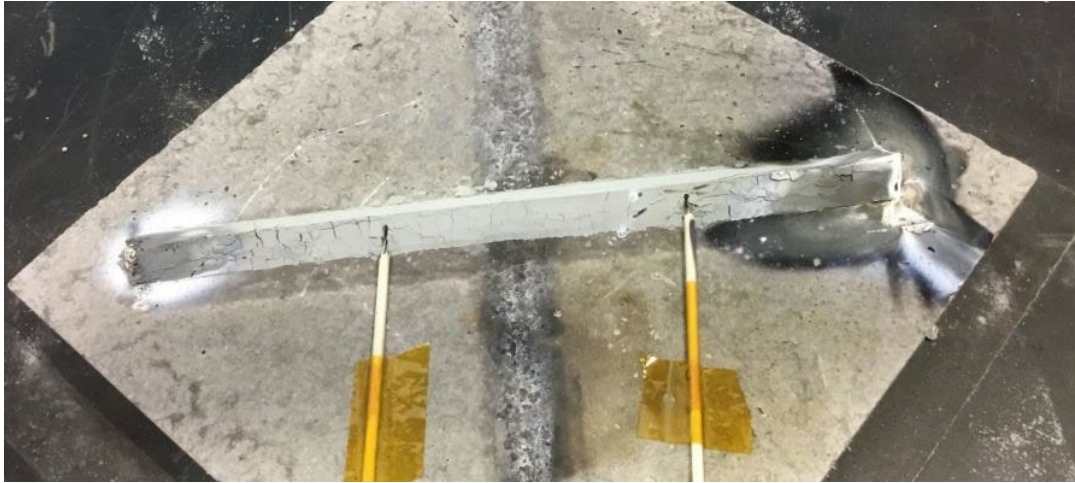
Figure A2-23 Zinc metal powder did not ignite when exposed to butane or propane-oxygen torch flames
