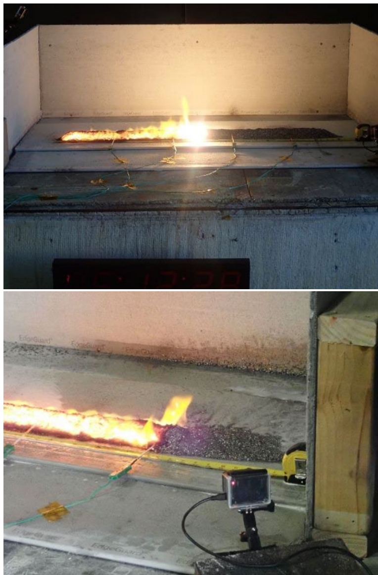
Figure A3-14 Titanium fines while burning (top) and after (bottom) F-500 was applied for 5 seconds
