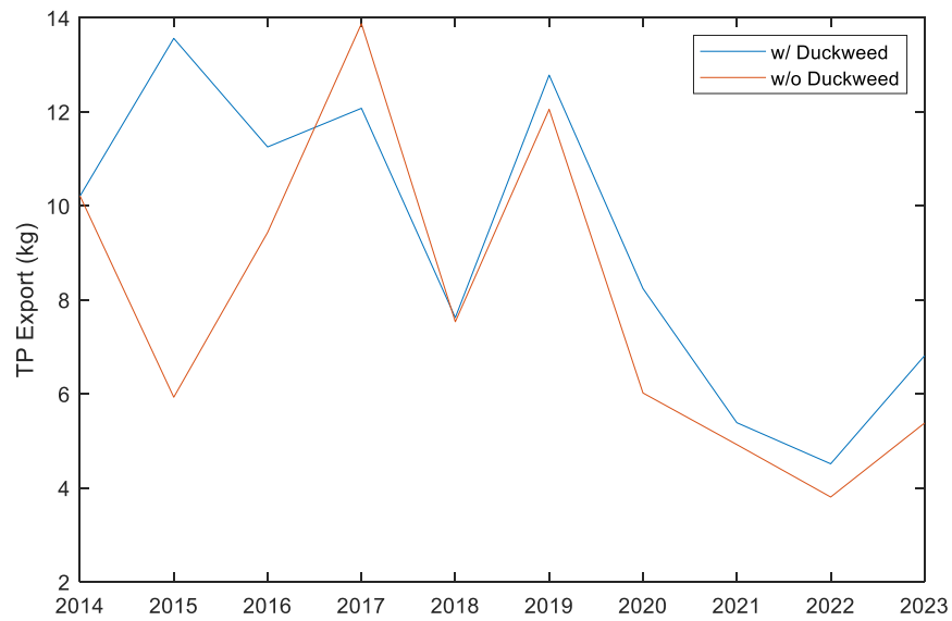
Figure 4-6. Simulated annual total phosphorus export from the Alameda historic wetland with and without duckweed growth.
