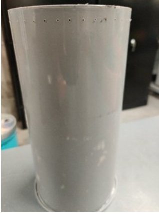
a) Predrilled mold (Upside down)
