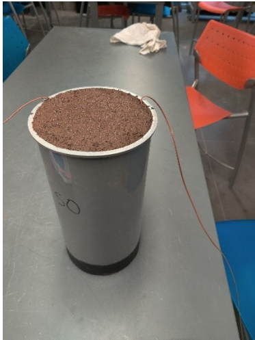
d) Compacted sample
