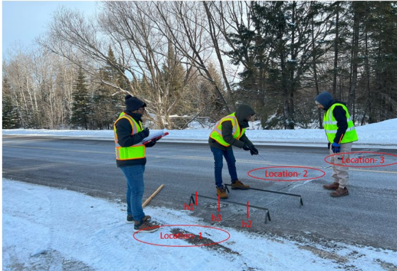
Figure 3.3 Tenting measuring device and the location of the measurements in a transverse crack
