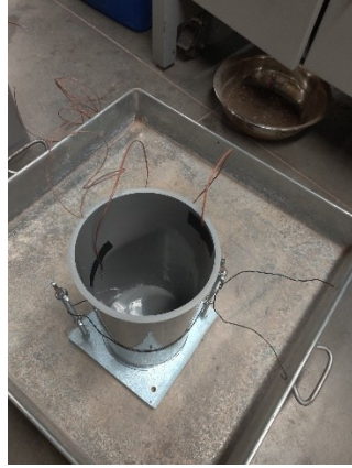
b) Thermocouple attached inside the PVC mold
