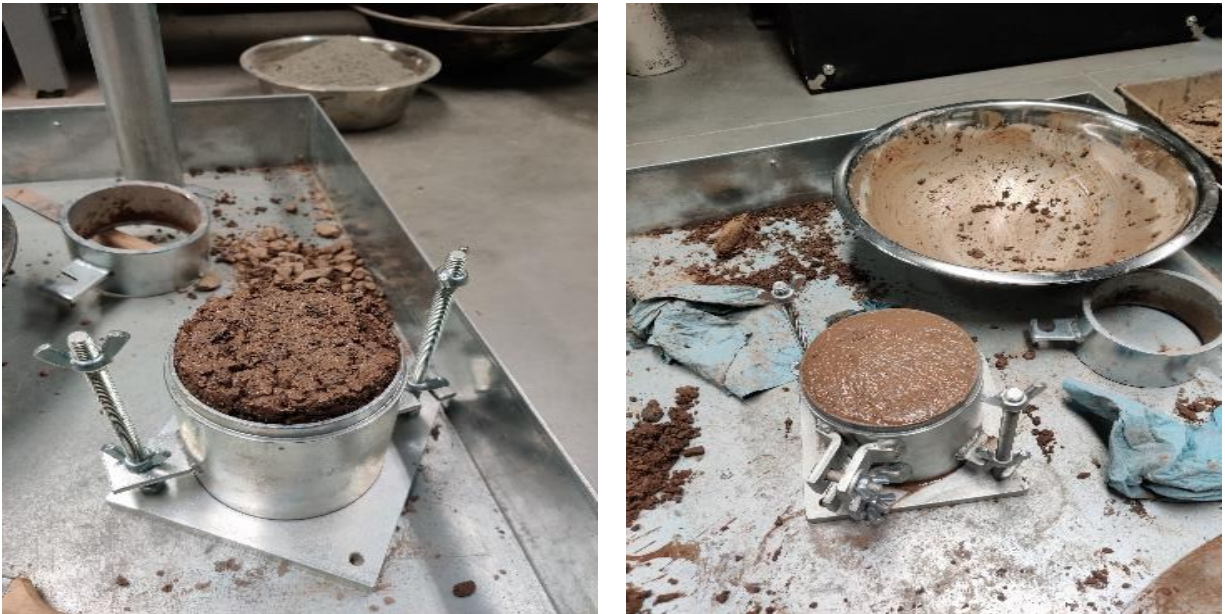
Figure 3.7 Photographs showing Proctor test of the base material
