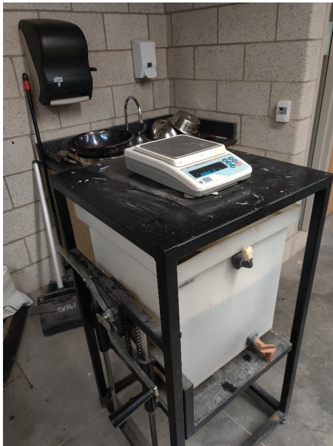
Figure 3.12 Coarse aggregate submerged in the water
