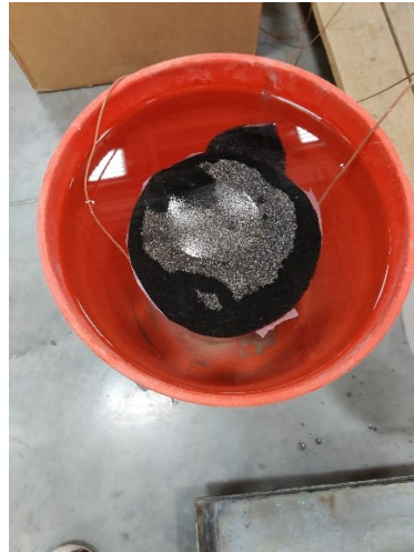
e) Sample saturation inside the water filled bucket
