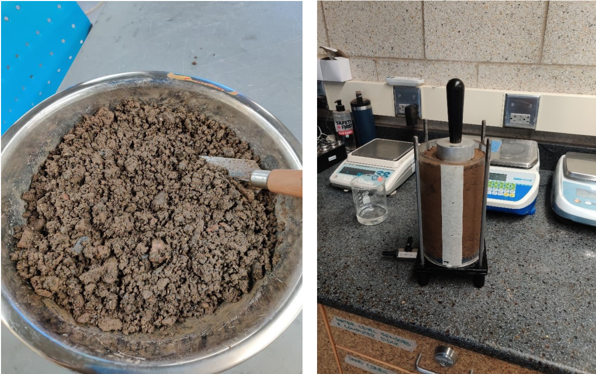
Figure 3.10 Aggregate mixed with water at OMC and Compacted sample in the permeability test mold.
