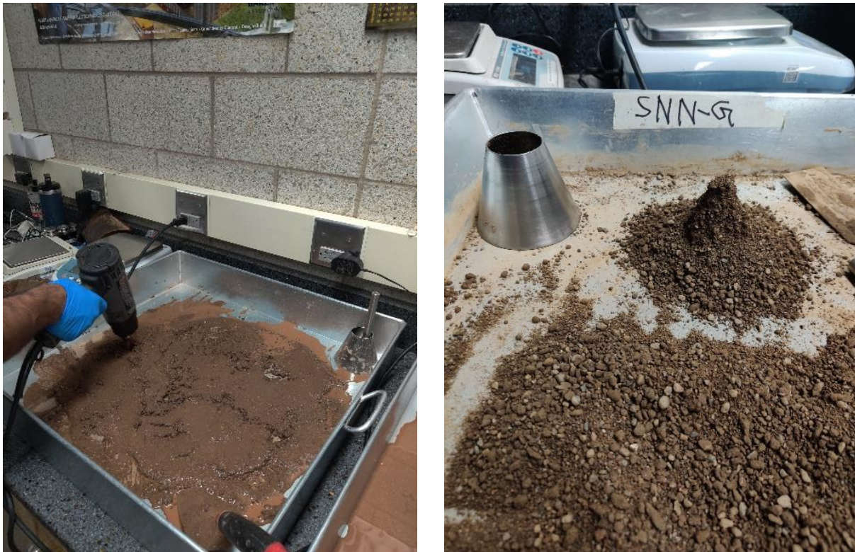
Figure 3.13 Fine aggregate drying using heat gun (left) and checking for SSD condition (right)
