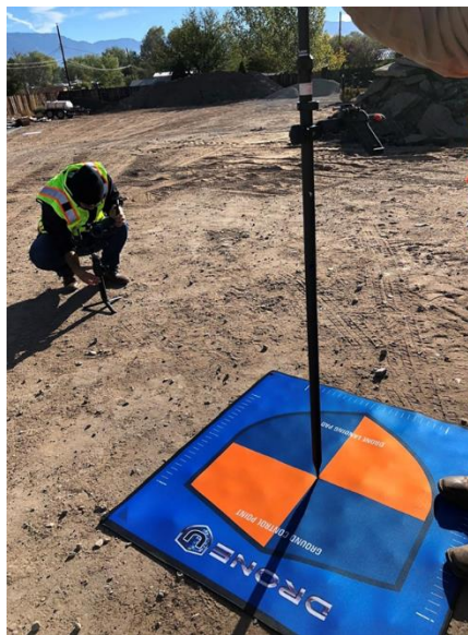
Figure 9. Sample surveying pad during field imaging
