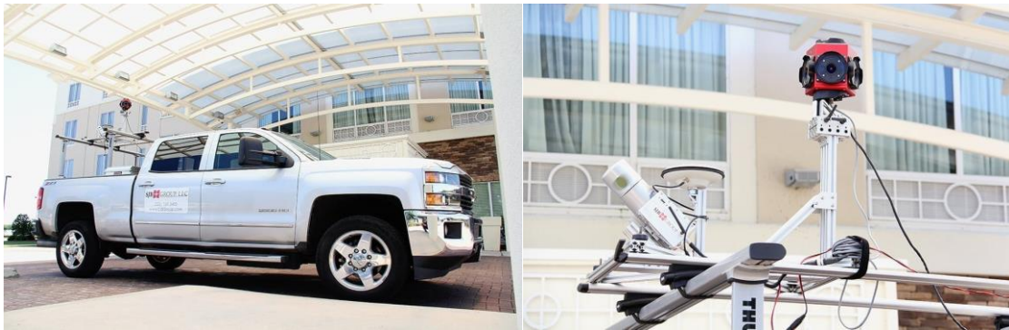
Figure 4. Vehicle used for DOTD’s LiDAR scanning as part of the I-20/I-220 Barksdale Air Force Base (BAFB) Interchange project in Bossier Parish [13]
