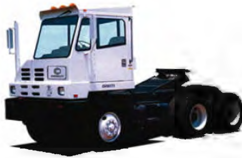
Exhibit 83: Powered Yard Tractor "Fifth Wheel"
