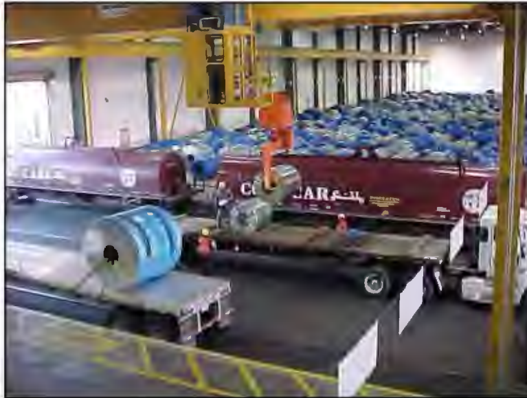
Exhibit 64: Coil Steel Transloading
