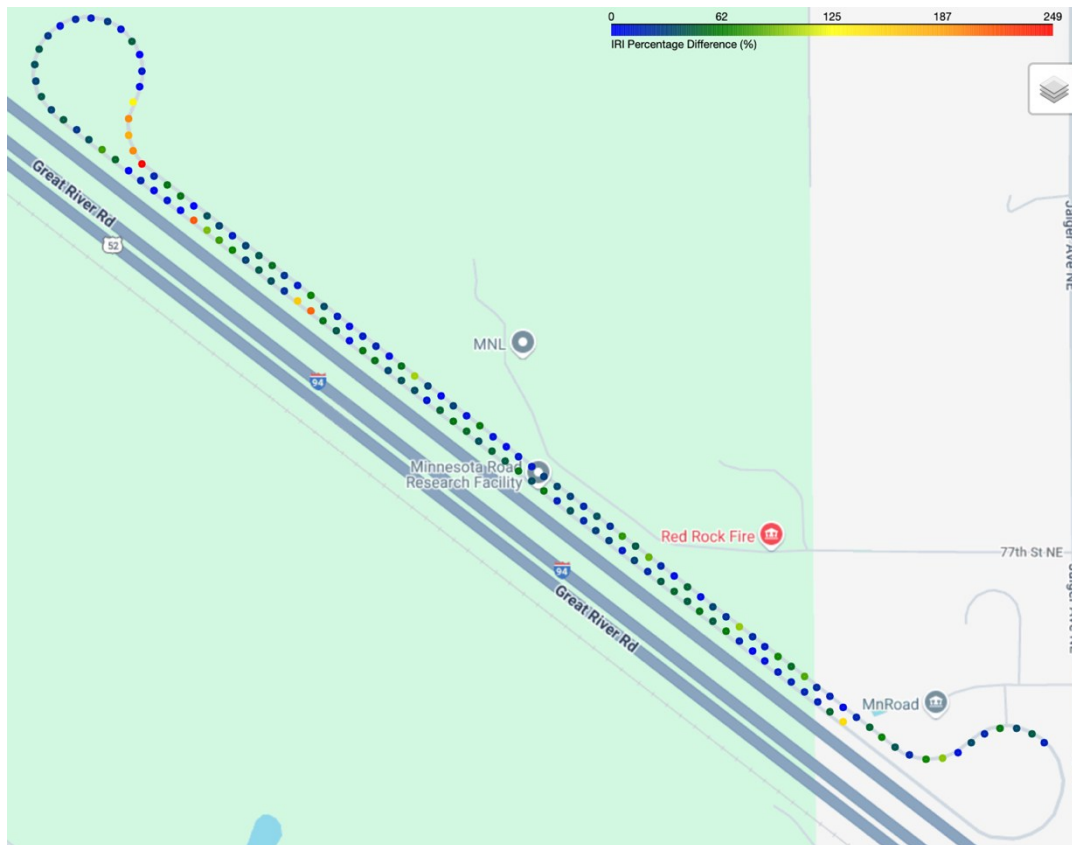
Figure 80. IRI percentage comparison between MnDOT ground truth measurements and Van collected data predictions for the MnROAD loop.
