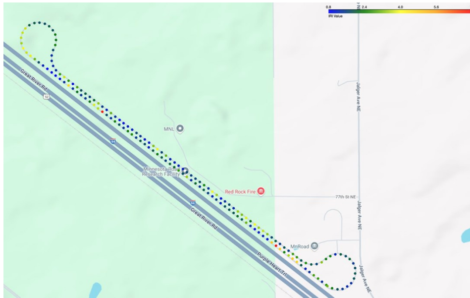
Figure 58. Color-coded visualization of true IRI measurements along the inside loop.
