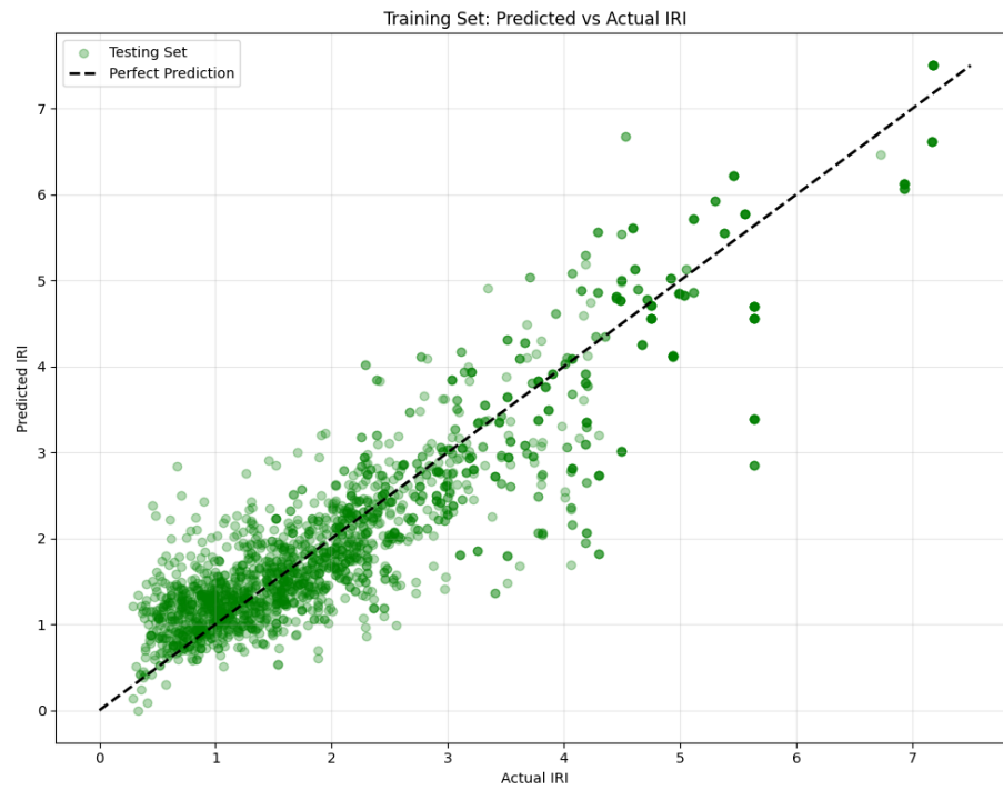
Figure 36. Predicted vs. actual IRI for SVR model testing set.
