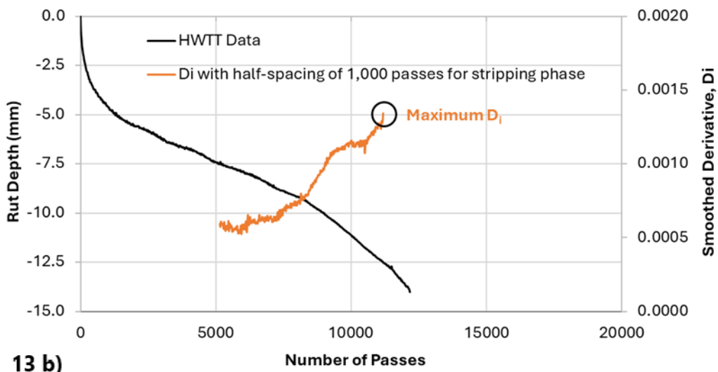
Figure 13. Determining Smoothed Derivative D_i for Method C: (a) using a Half-spacing of 2,000 Passes for Creep Phase, (b) using a Half-spacing of 1,000 Passes for Stripping Phase
