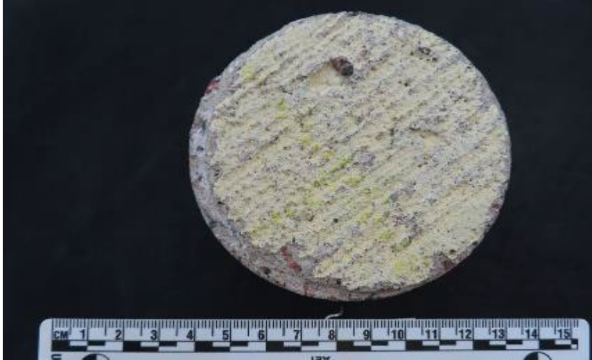
Figure 5.3 The drag textured top surface bearing AMS curing compound as received. MnROAD Core sample 243725CC01 Description: Profile of the core sample as received with the top surface to the left.
