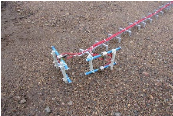
Figure 3.5 Vibrating wire strain gauges
