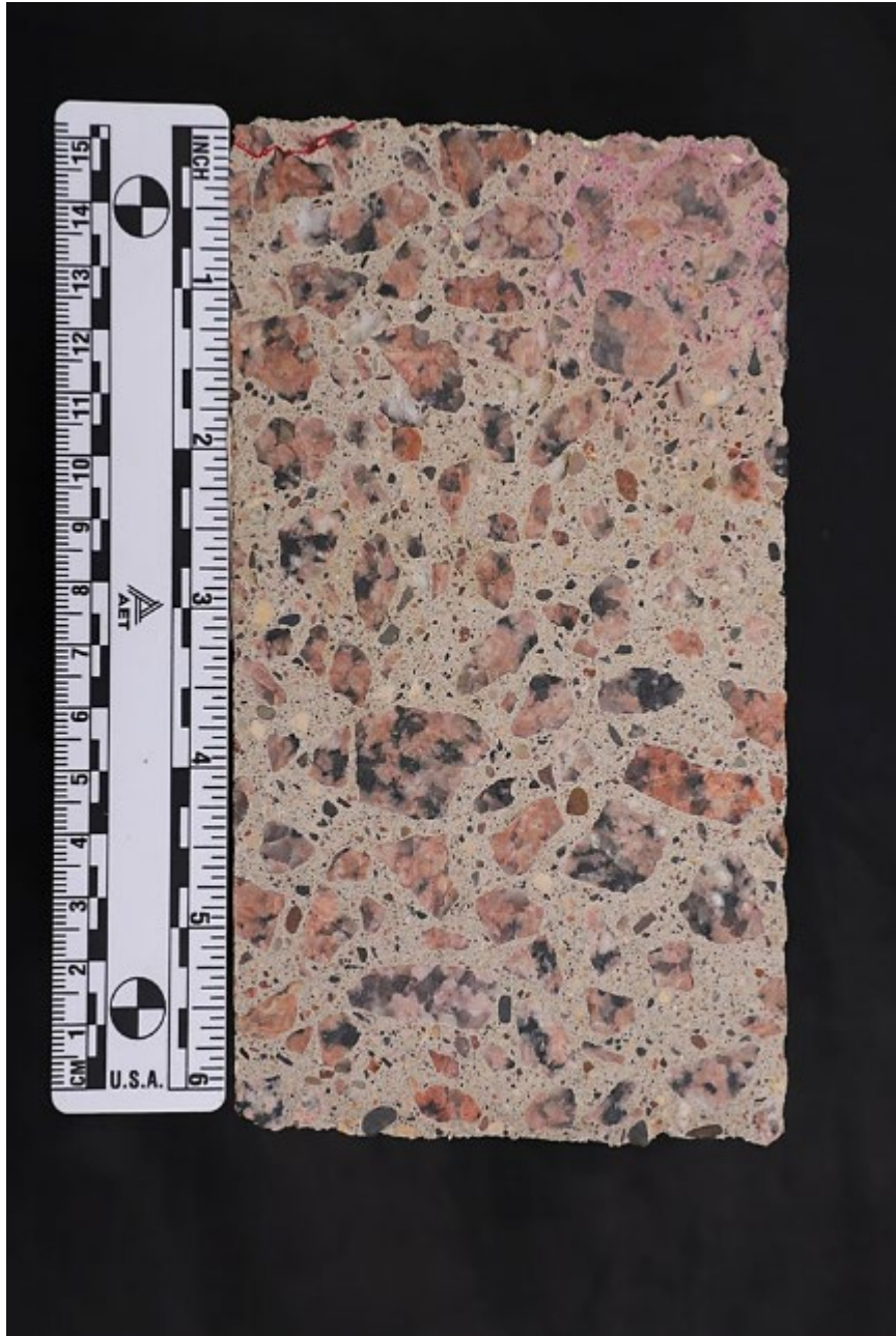
Figure 5.4: Saw cut and lapped cross section with the top surface oriented to the top of the photo.
