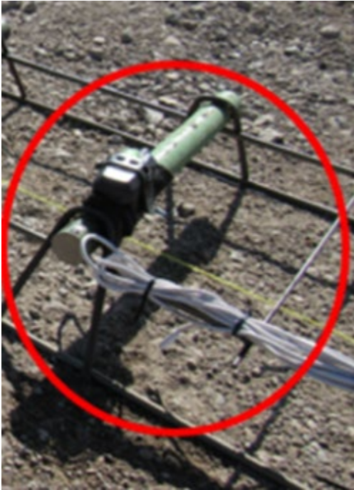
Figure 3.4 Typical instrumentation location for maturity sensor
