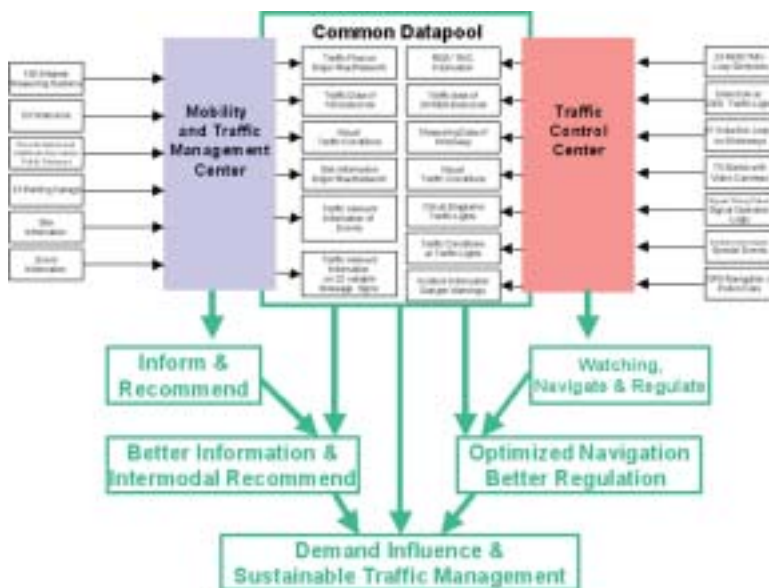
Figure 34. Cooperation in the traffic management center.
