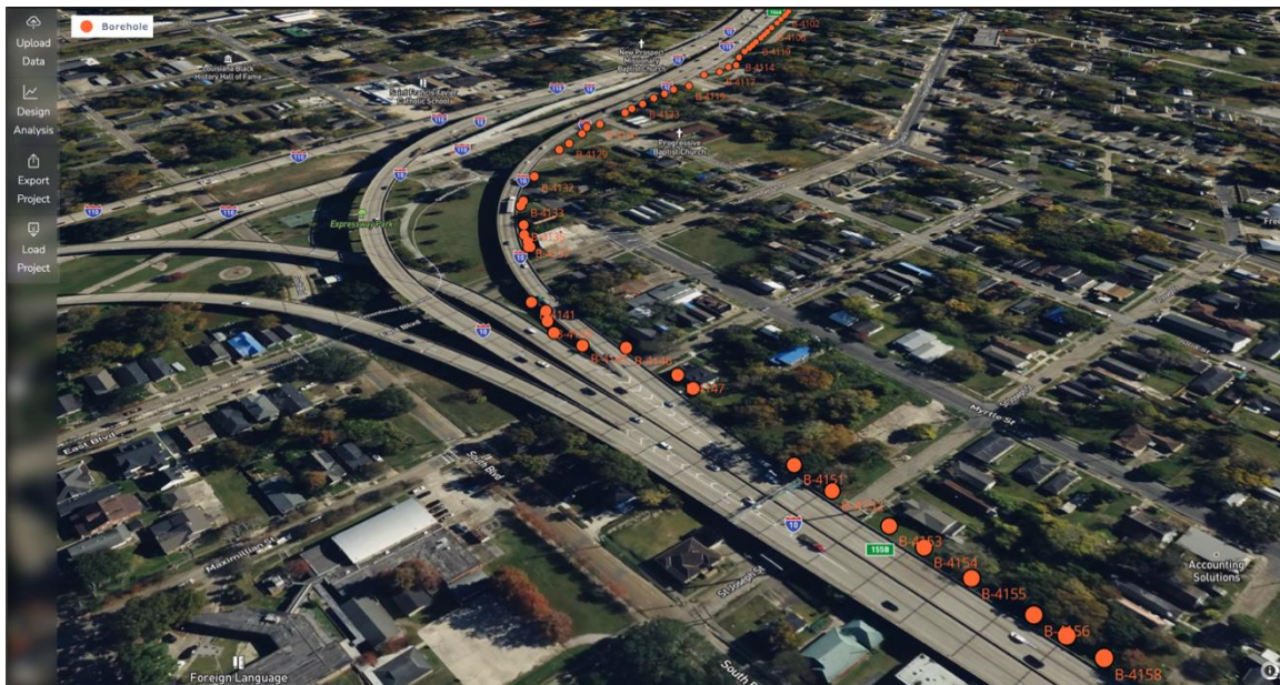
Figure 14. 3-D interactive map view displaying deep soil boring locations imported from a gINT file onto the web-based platform
