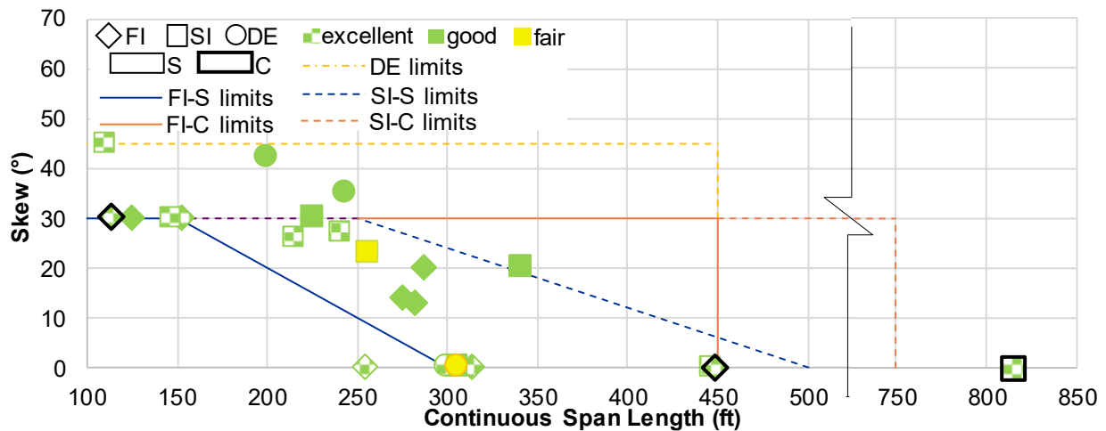
Figure 22. Visual Condition of Surveyed Abutment Backwalls for Given Continuous Span Length and Skew. C = concrete superstructure; DE = deck extension; FI = full integral; S = steel superstructure; SI = semi-integral.
