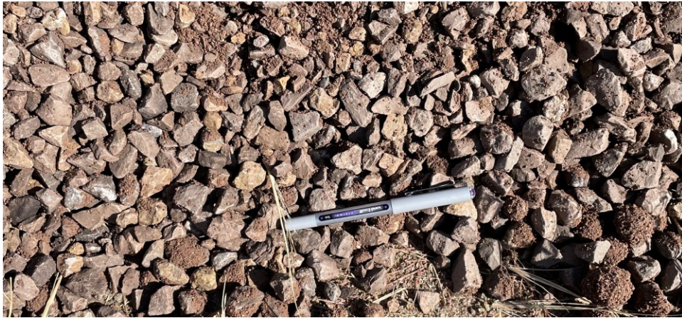
Figure 4.3 Mixed treatment media, showing clay, fine (sand sized) aggregate and coarse aggregate mixed together (pen for scale).
