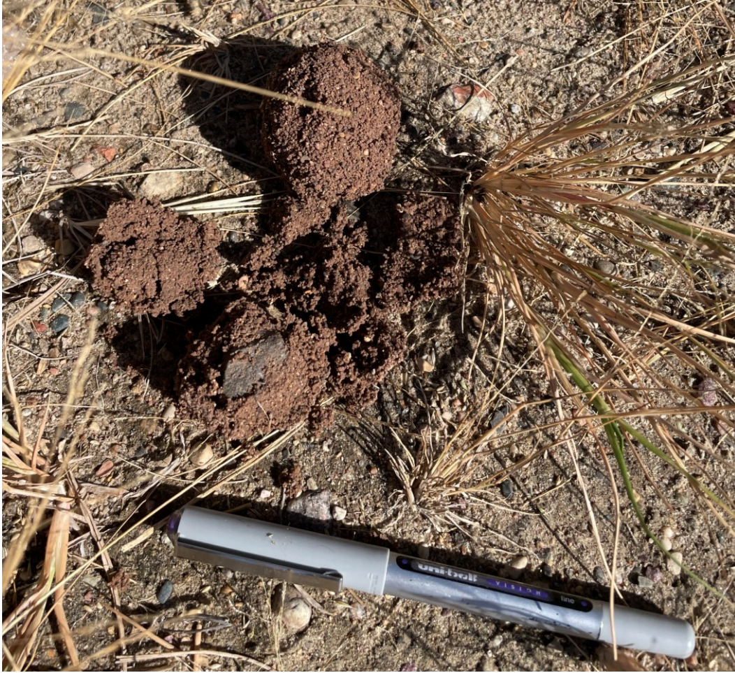
Figure 4.4 Armored clay balls created during the mixing process (pen for scale).
