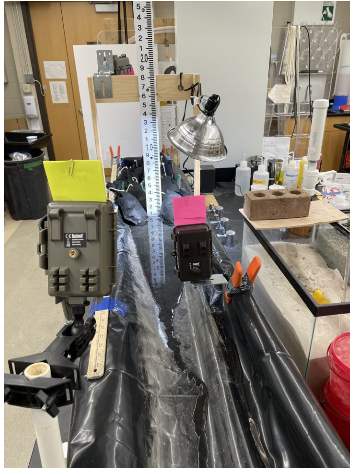
Figure 3.2 Waterway channel in operation with flowing water modeling snow and ice melt-out, treatment media flow-through bags in channel, water ponded behind bags, stream staff gage for depth measurement, light, and time lapse cameras.
