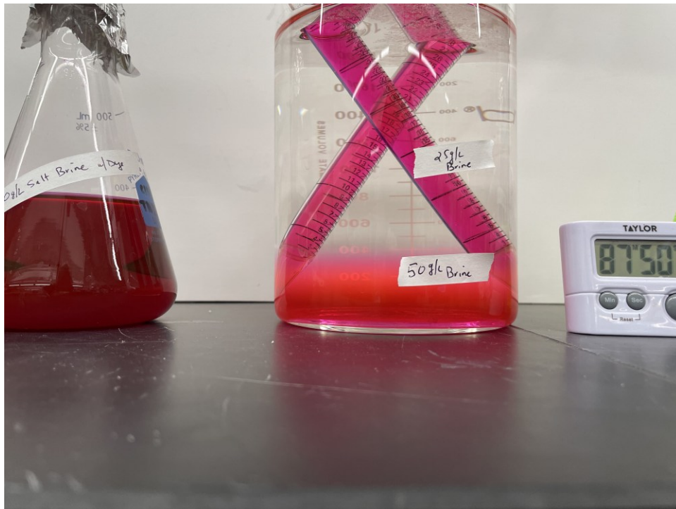
Figure 3.11 Density 2 days after brine injection.
