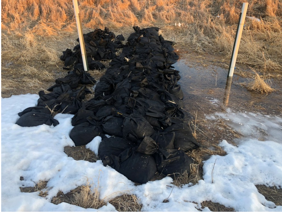
Figure 4.16 Ditch water flowing through the treatment berm during melt out; Sterling South location, March 11, 2025. Flow from right to left.
