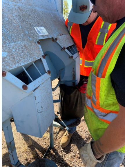
Figure 4.6 Treatment bag filling by hand (top) and sandbag filler with hopper and auger system (bottom)
