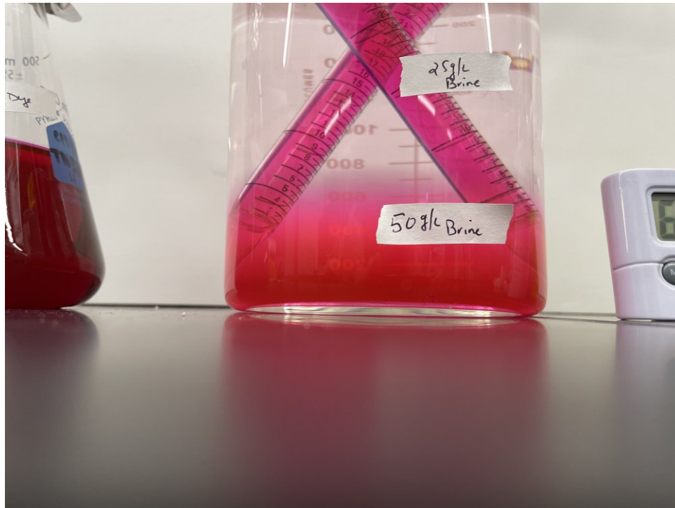
Figure 3.12 Density 5 days after brine injection
