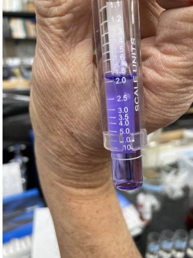
Figure 2.8 A vacu-vial reverse titration analysis with purple-colored fluid currently reading 2% chloride; additional sample titration into the vial will cause the purple color to turn colorless signifying the actual concentration of chloride in the sample
