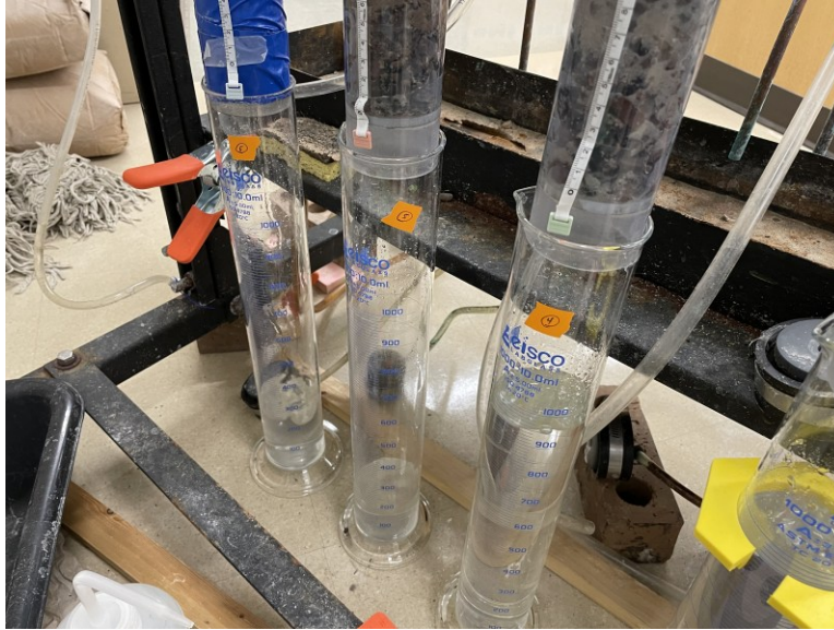
Figure 2.6 Graduated cylinders receiving treated effluent water beneath the columns.
