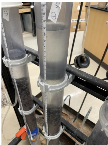
Figure 2.7 Falling head permeability tests being conducted above and through filter packs with brine fluid in Column 5 at 60.6 cm (foreground) and in Column 6 at 49.8 cm (background).
