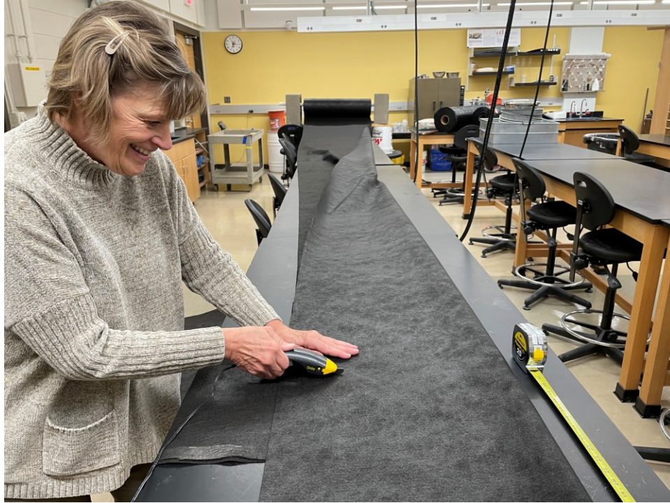
Figure 4.5 Geotextile cutting, the first step in making flow-through bags.
