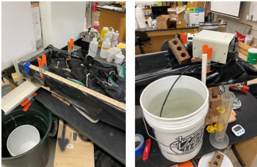
Figure 3.4 Waterway lower (discharge) end (left, with treatment bags, discharge gutter and receiving bucket) and upper (in-flow) end (right, with reservoir bucket, pump, and in-channel brick for holding the pump tubing)
